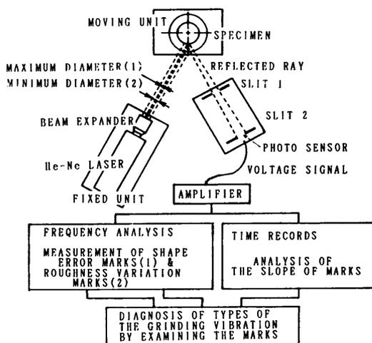
Fig. 3 Outline of measurement and analysis of light reflectivity variation for grinding marks
