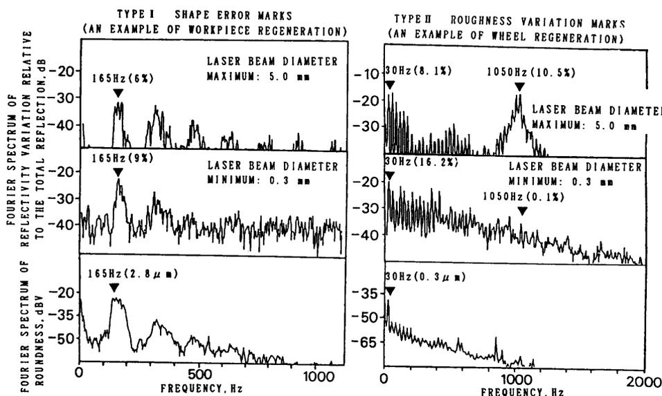
Here the percent values in the parentheses indicate power spectrum ratio of the noted frequency component to all components below 1 000 Hz (left) and below 2 000 Hz (right)
