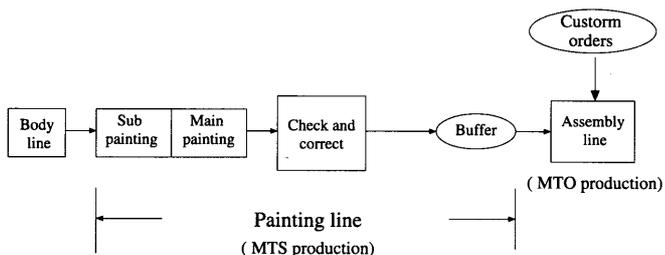
Fig. 2 Scheme of the painting line model
