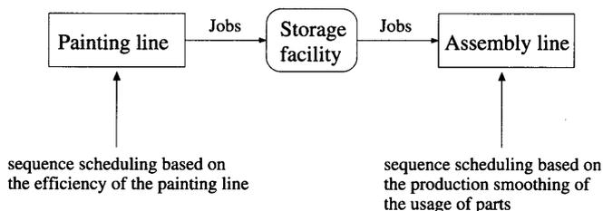
Fig. 1 Scheme of the sequencing method by Monden
