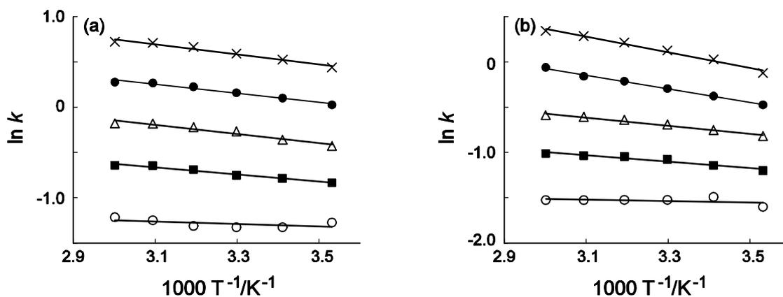
**Figure 3-3-2** van't Hoff plots for pyrazines with (B) ACN/water = 30/70 as the mobile phase on two types of bonded stationary phases. Stationary phase: (a) Inertsil ODS-3 (5  $\mu$ m, 150 mm x 4.6 mm i.d.), (b) Inertsil C8-3 (5  $\mu$ m, 150 mm x 4.6 mm i.d.). Other chromatographic conditions and the peak assignments are the same as in Fig. 3-2.
