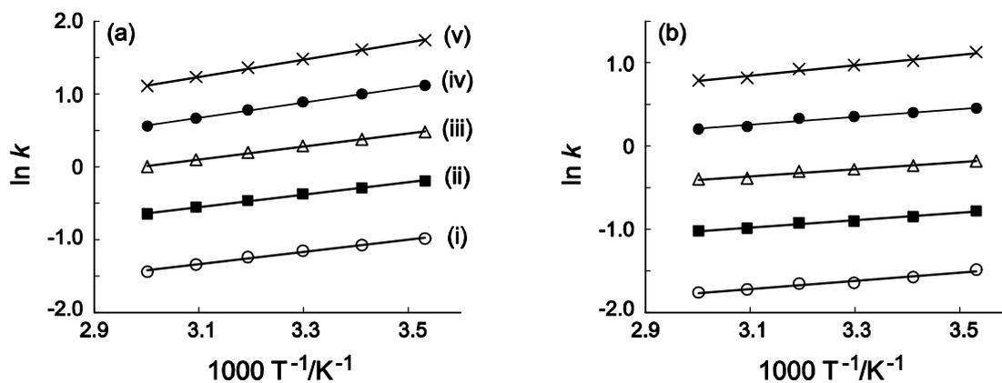
**Figure 3-3-1** van't Hoff plots for pyrazines with MeOH/water = 40/60 as the mobile phase on two types of bonded stationary phases. Stationary phase: (a) Inertsil ODS-3 (5  $\mu$ m, 150 mm x 4.6 mm i.d.), (b) Inertsil C8-3 (5  $\mu$ m, 150 mm x 4.6 mm i.d.). Other chromatographic conditions and the peak assignments are the same as in Fig. 3-2.
