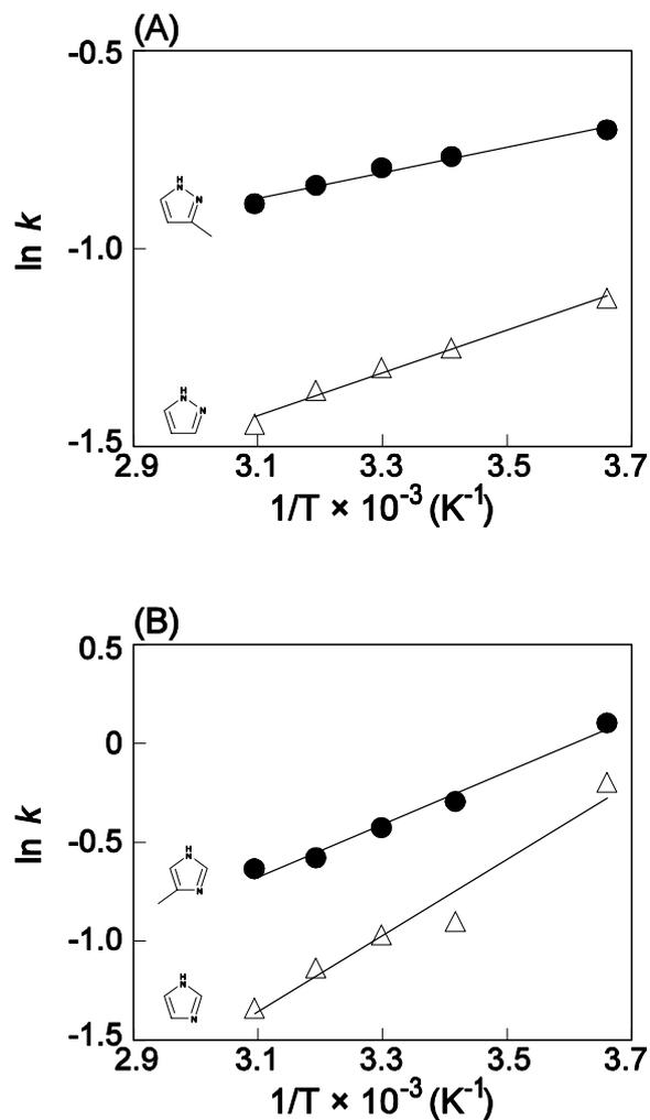
**Figure 4-6** van't Hoff plots for pyrazoles and imidazoles. Mobile phase: ACN/water = 30/70. Analyte: (A) pyrazoles and (B) imidazoles. Other conditions are the same in Figure 4-3.
