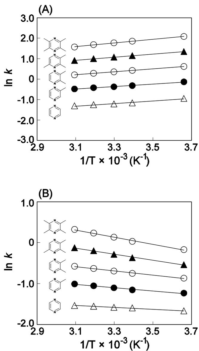
**Figure 4-3** van't Hoff plots for pyrazines. Mobile phase: (A) MeOH/water = 30/70; (B) ACN/water = 30/70. Other conditions are the same in Figure 4-2; and the assignments are the same as in Figure 4-1.
