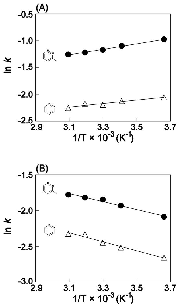
**Figure 4-4** van't Hoff plots for pyridazine and 3-methylpyridazine. Mobile phase: (A) MeOH/water = 30/70; (B) ACN/water = 30/70. Other conditions are the same in Figure 4-3.
