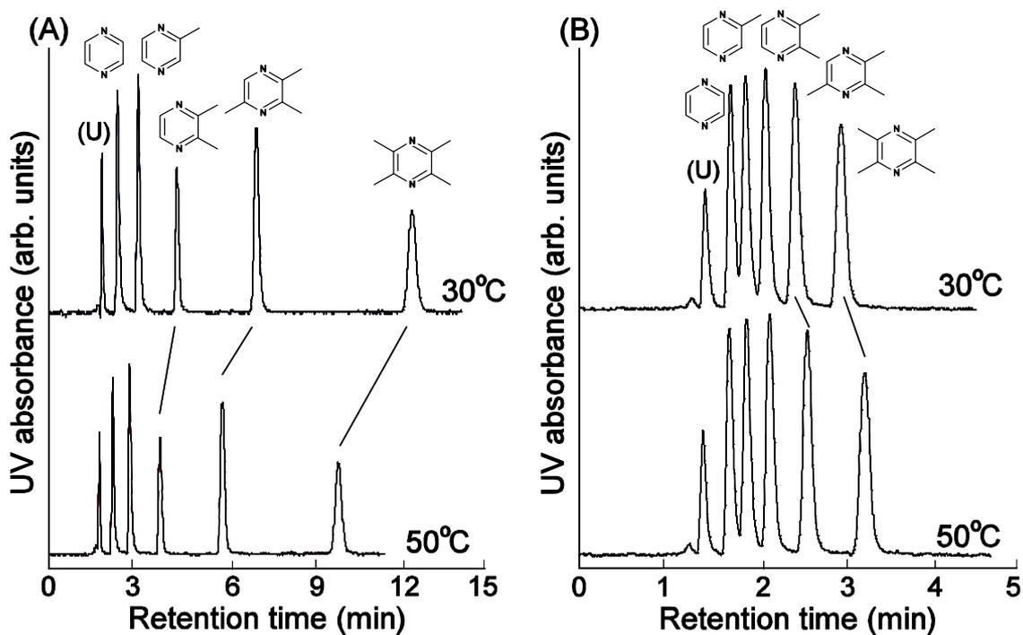
**Figure 4-2** Typical chromatograms for the separation of pyrazines at different column temperatures. Mobile phase: (A) MeOH/water = 30/70; (B) ACN/water = 30/70. As dead volume marker, uracil (U) was used. Other conditions: column, ULTRON VX-ODS (5 $\mu$ m, 150 mm x 4.6 mm i.d.); flowrate, 1.0 mL/min; detection, UV at 270 nm.
