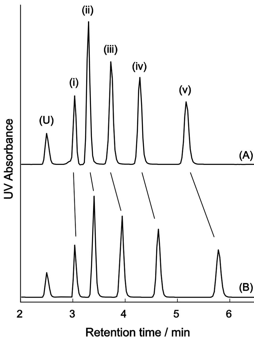
**Figure 3-2** Typical chromatograms for the separation of pyrazine and alkympyrazines at different column temperatures. (A) 30°C and (B) 60°C. Other conditions: column, Inertsil ODS-3 (5  $\mu$ m, 150 mm x 4.6 mm i.d.); mobile phase, ACN/water = 30/70, flowrate, 0.6 mL/min; detection, UV at 270 nm. Peaks: (U) uracil, (i) pyrazine, (ii) 2-methylpyrazine, (iii) 2,3-dimethylpyrazine, (iv) 2,3,5-trimethylpyrazine, (v) 2,3,5,6-tetramethylpyrazine.
