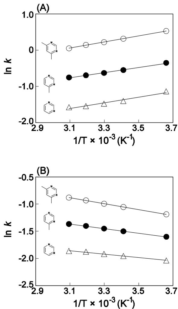
**Figure 4-5** van't Hoff plots for pyrimidine, 4-methylpyrimidine and 4,6-dimethylpyrimidine. Mobile phase: (A) MeOH/water = 30/70; (B) ACN/water = 30/70. Other conditions are the same in Figure 4-3.
