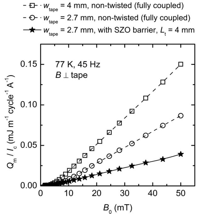
Figure 4 Normalized AC losses  $Q_m/I_c$  at 77 K and 45 Hz for twisted barrier tape with  $L_t = 4 \text{ mm}$ . The data for non-twisted tapes with tape width of 4 mm and 2.7 mm are also plotted as the references
