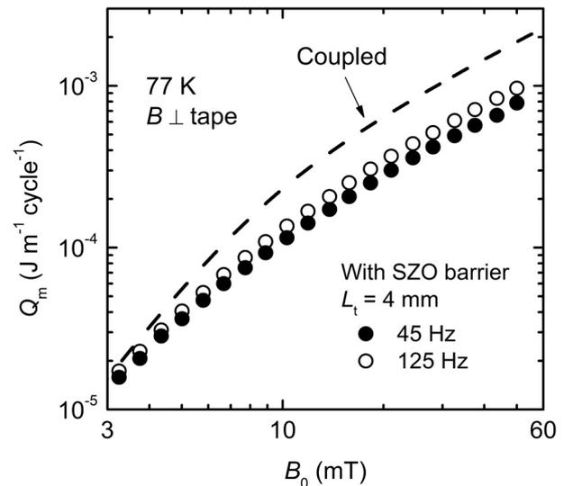
Figure 5 AC losses  $Q_m$  per-cycle at 45 Hz and 125 Hz for twisted tape with SZO barriers ( $L_t = 4 \text{ mm}$ ), plotted against perpendicular field amplitude  $B_0$ . A dashed line represents a prediction for a tape with fully coupled filaments.
