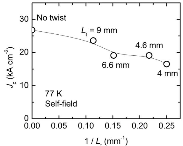
Figure 2 Self-field  $J_c$  at 77 K for Bi2223 tapes with SZO barriers plotted against inverse of twist lengths  $L_t$
