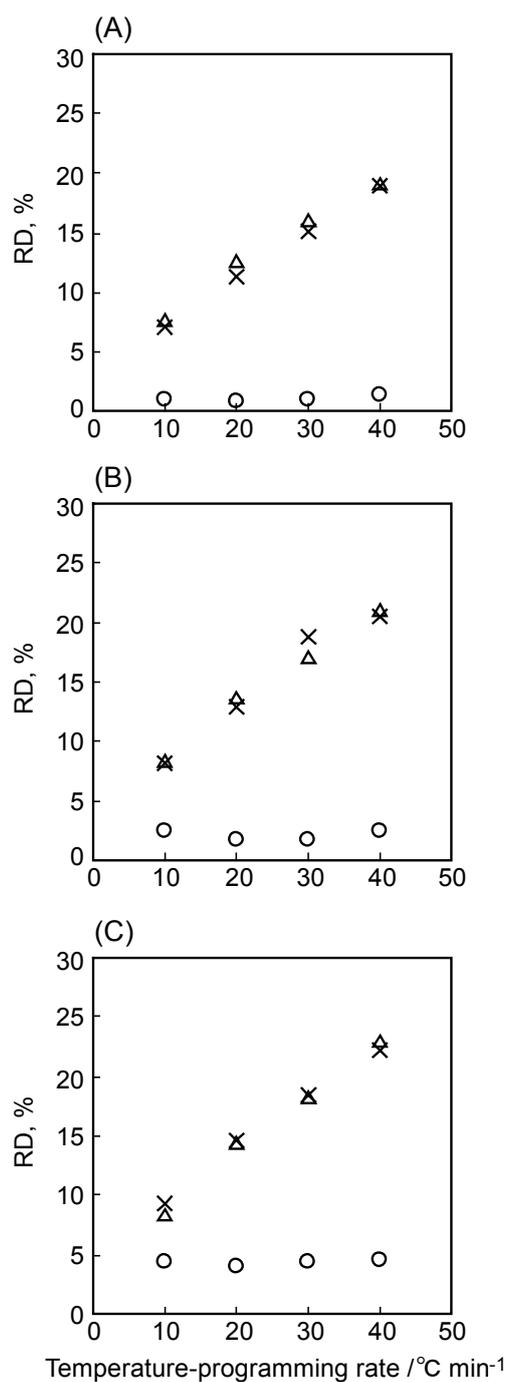
**Figure 2-2** Relative delay of the actual retention time from that estimated for various separation conditions.
