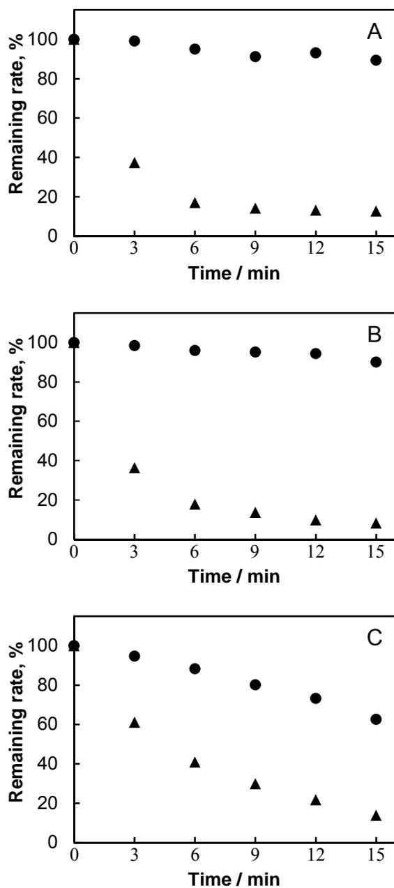
**Figure 5-3** Time profile of VOCs concentration in the sample vial with (triangle) and without (circle) polyimide particles. (A) acetone, (B) hexane and (C) toluene.
