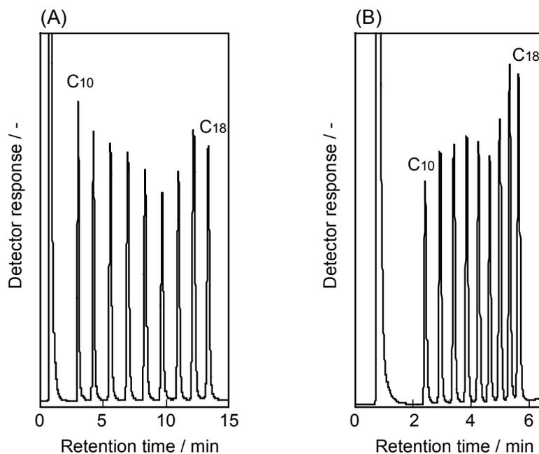
**Figure 2-3** Chromatograms for the separation of alkanes on the developed packed-capillary column at different temperature programs. Temperature program: (A) 100°C (1 min) to 240°C at a rate of 10°C/min; (B) 100°C (1 min) to 300°C at a rate of 40°C/min. Detector, FID at 300°C; column head pressure, 70 kPa; injection, splitless injection of 1.0 L; sample, alkane mixture containing 1.0% each of nine alkanes from decane to octadecane in hexane as the solvent.
