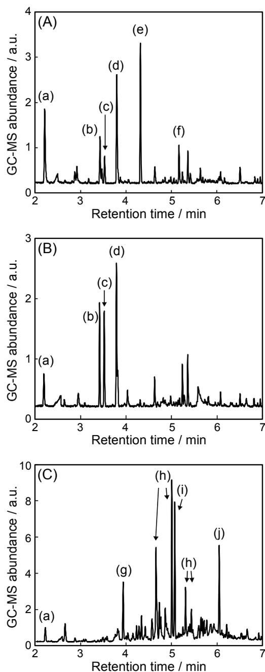
**Figure 3-3** Typical chromatograms for the separation of VOCs found in large-scale repaired school facilities (school B).
