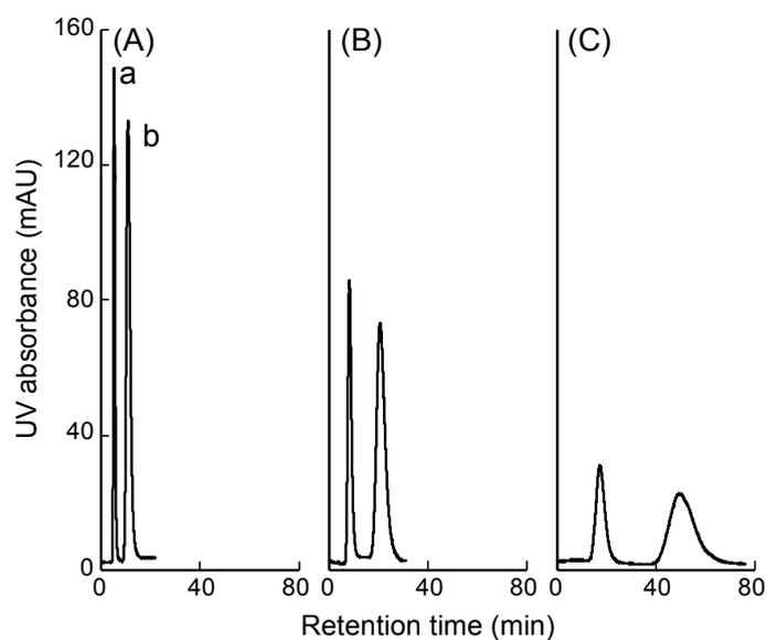
**Figure 4-5** Separation of o-terphenyl and triphenylene on the crosslinked chitosan phase (DCC-1) with different mobile phase compositions. Mobile phase composition (methanol/water): (A) 90/10; (B) 80/20; and (C) 70/30. Other conditions are in the text. Peaks: (a) o-terphenyl; (b) triphenylene.
