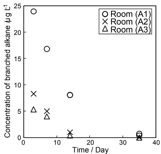
**Figure 3-2** Time profile of a branched alkane found in in-room air samples after a renovation in school A.
