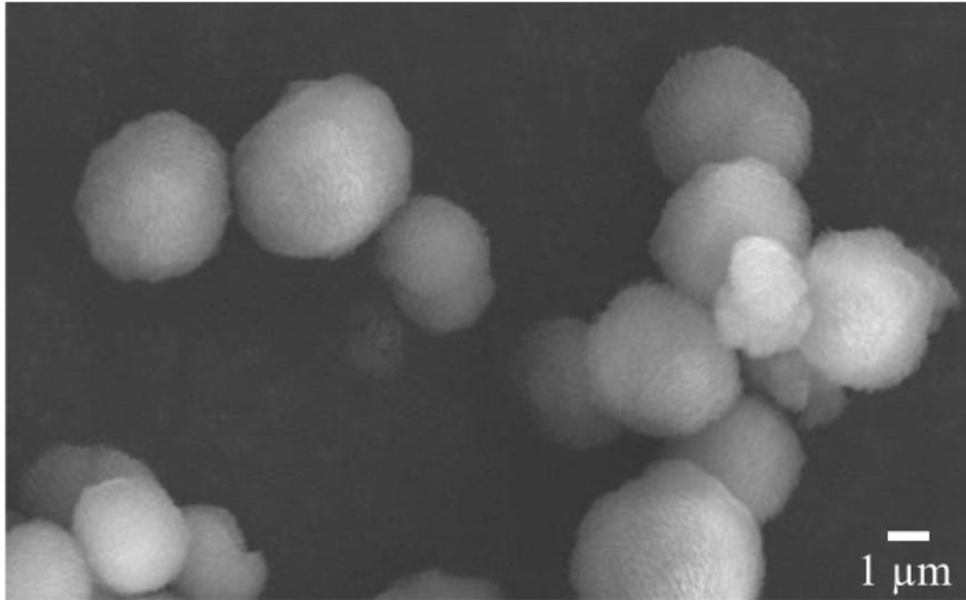
**Figure 5-2** SEM image of the PMDA-ODA particles.
