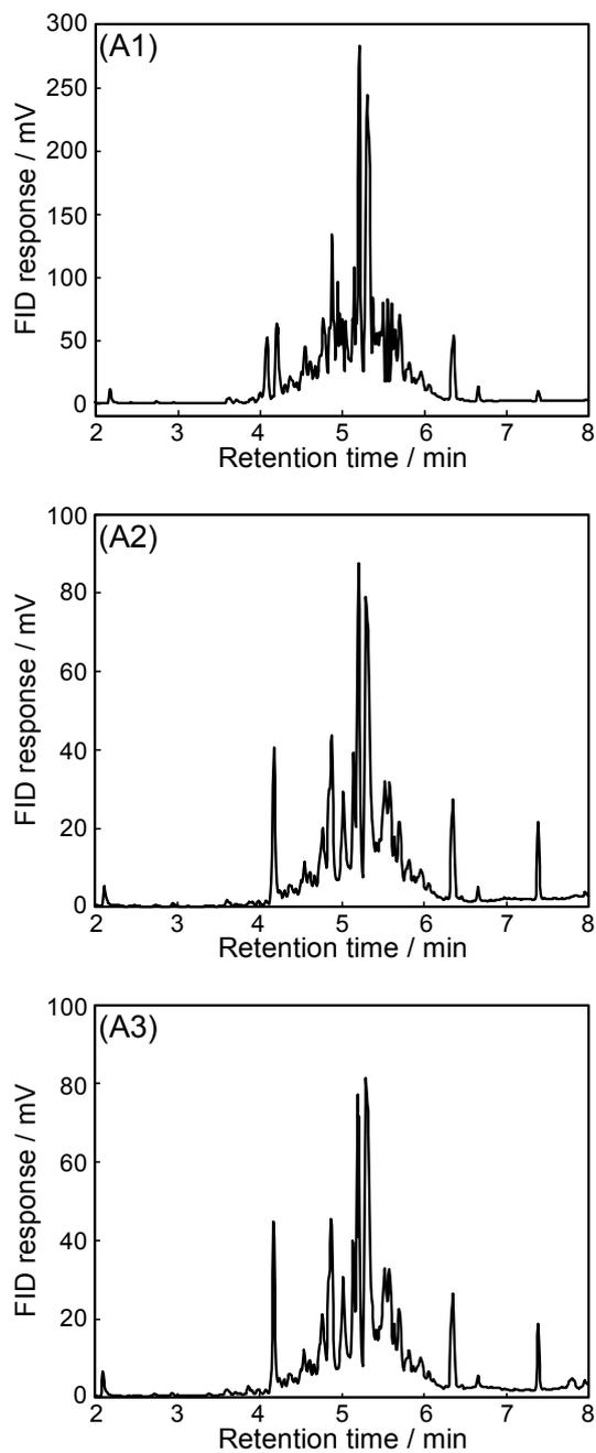
**Figure 3-1** Chromatograms for the separation of branched alkanes observed in three small teachers' rooms after a renovation in school A.
