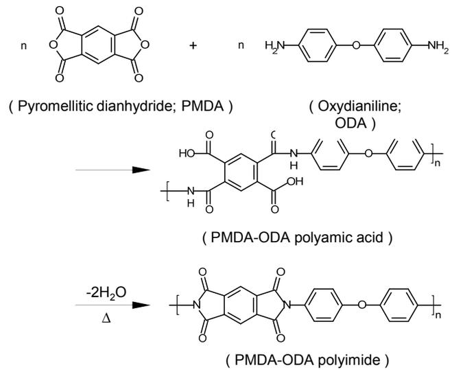
**Figure 5-1** Synthetic scheme of PMDA-ODA.
