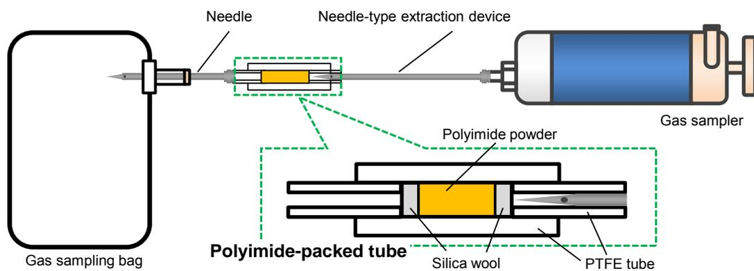
**Figure 5-4** Illustration of polyimide-packed tube and experimental setup for the evaluation of the dynamic sampling/extraction.
