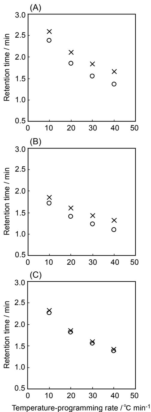
**Figure 2-1** Comparison of the measured (cross) retention data with that estimated (open circle) for three types of packed columns using temperature-programmed analyses at different ramp rates.
