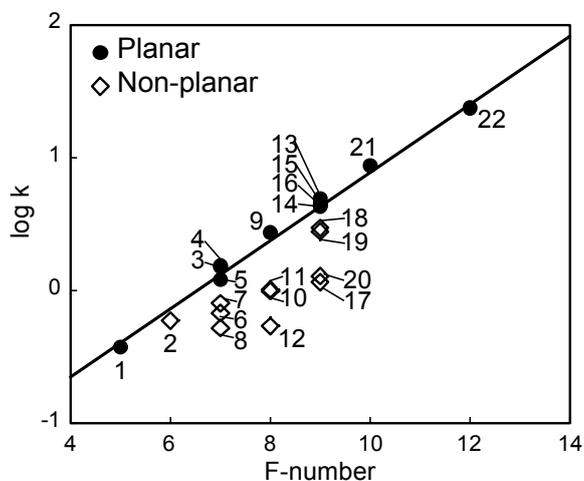
**Figure 4-4** Relationship between logarithmic retention factor ( $\log k$ ) and  $F$ -number for various PAHs with the crosslinked chitosan phase (DCC-1). Conditions are the same as in Figure 3, except for the detection wavelength for perylene and coronene at 300 nm. All the solute assignments are the same as in Figure 2.
