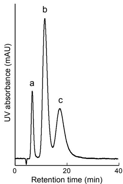
**Figure 4-3** Typical chromatogram of PAHs on the crosslinked chitosan stationary phase (DCC-1). Conditions: mobile phase, methanol/water = (80/20); detection wavelength, 254 nm. Other conditions are found in the text. Peaks: (a) naphthalene; (b) anthracene; (c) pyrene.
