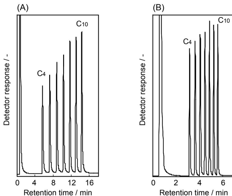
**Figure 2-4** Typical chromatograms for the separation of seven alkylbenzenes from butylbenzene (C4) to decylbenzene (C10) on the packed-capillary column.
