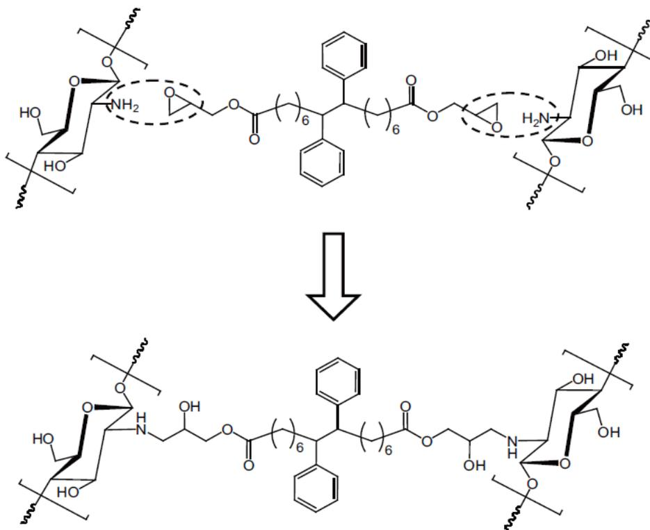
**Figure 4-1** Synthetic scheme of crosslinked chitosan stationary phase.
