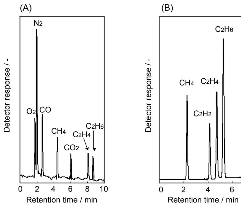
**Figure 2-5** Rapid temperature-programmed separations on the packed-capillary column. Stationary phase, Shincarbon ST; column size, 1.0 mm i.d. x 2.0 m length.
