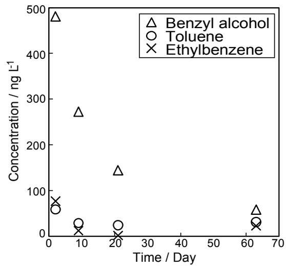
**Figure 3-4** Time variations of three VOCs after a large-scale repair in class room B3.
