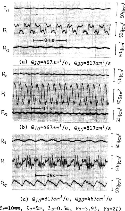
Fig.7 Examples of the wave forms for the double-capacity-oscillator obtained from the experiments
