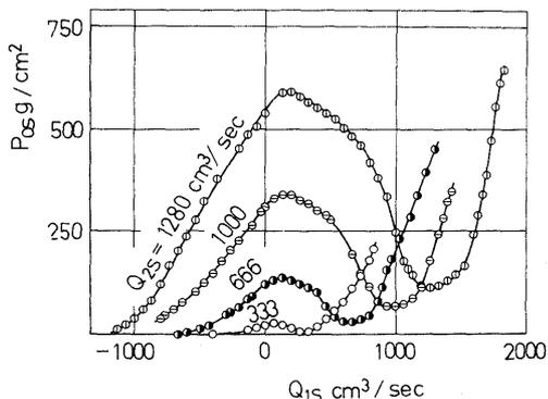
Fig.2 Steady state characteristics of the vortex valve
