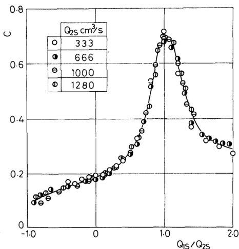
Fig.3 Discharge coefficient of the valve outlet orifice
