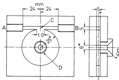
Fig.1 Shape and dimensions of test vortex valve
