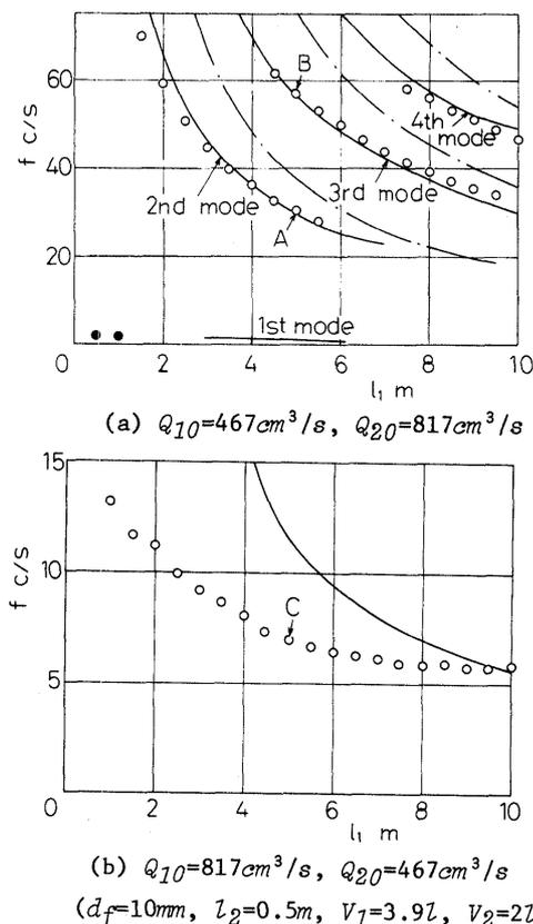
Fig.8 Frequencies of the oscillation for the double-capacity-oscillator
