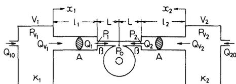
Fig.4 Schematic diagram of the confined vortex oscillator
