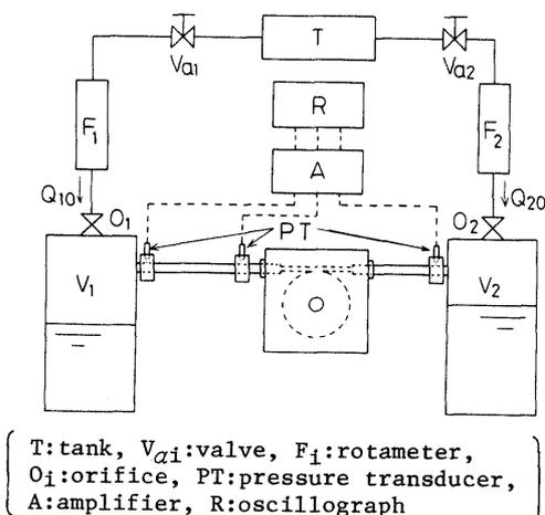
Fig.6 Schematic diagram of the experimental apparatus
