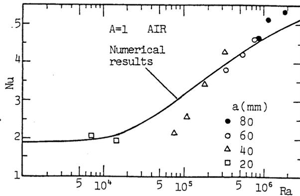
Fig.14 Oscillating flow and heat transfer coefficient
