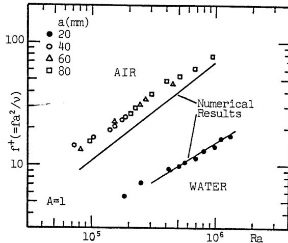
Fig.10 Non-dimensional frequency for periodically oscillating flow
