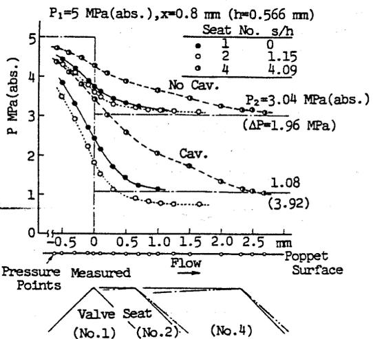
Fig.10 Pressure distribution on the poppet surface (converging flow)
