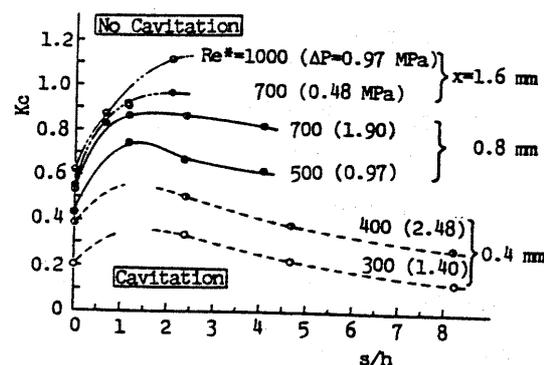
Fig. 12 Critical cavitation number for the inception (diverging flow)
