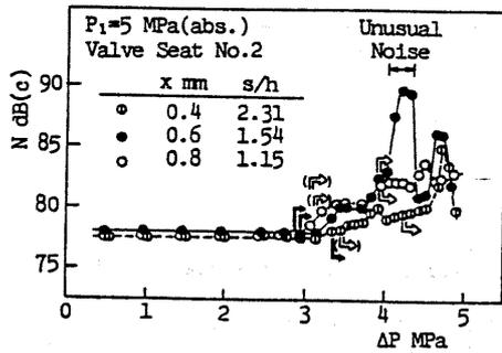
Fig.14 Noise performance (diverging flow, valve seat No.2)
