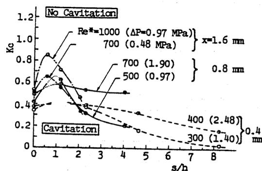
Fig. 13 Critical cavitation number for the inception (converging flow)
