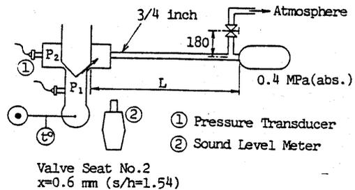
Fig.16 Schematic diagram of apparatus for the examination of unusual sound
