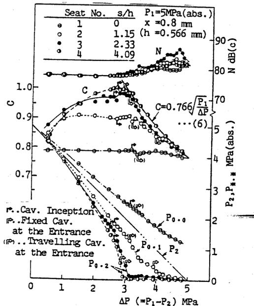
Fig.3 Flow characteristics (diverging flow)
