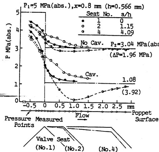
Fig.5 Pressure distribution on the poppet surface (diverging flow)
