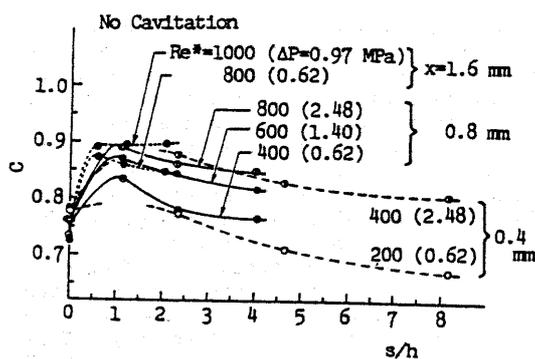
Fig. 11 Discharge coefficient versus  $S/h$  (converging flow)
