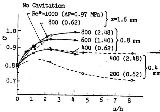
Fig.6 Discharge coefficient versus  $S/h$  (diverging flow)
