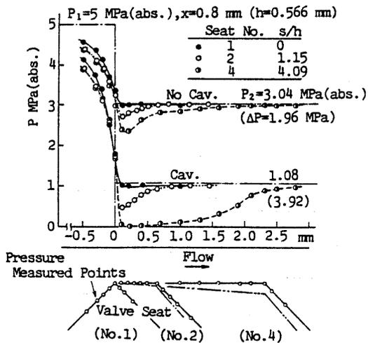
Fig.4 Pressure distribution on the valve seat (diverging flow)
