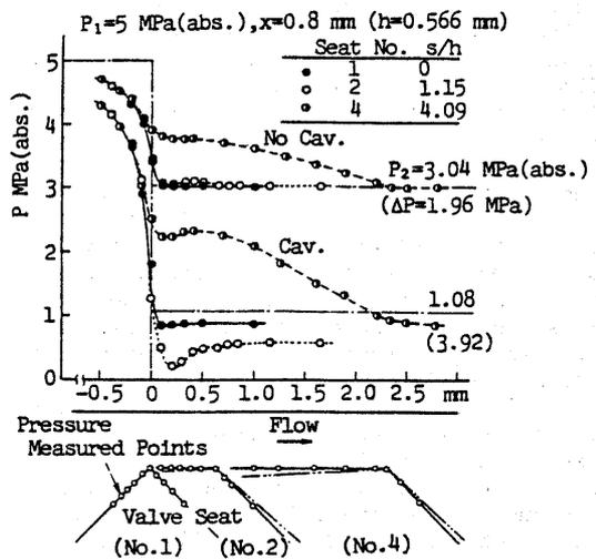
Fig.9 Pressure distribution on the valve seat (converging flow)
