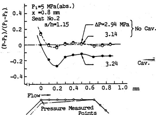
Fig.8 Change of pressure distribution with occurrence of cavitation
