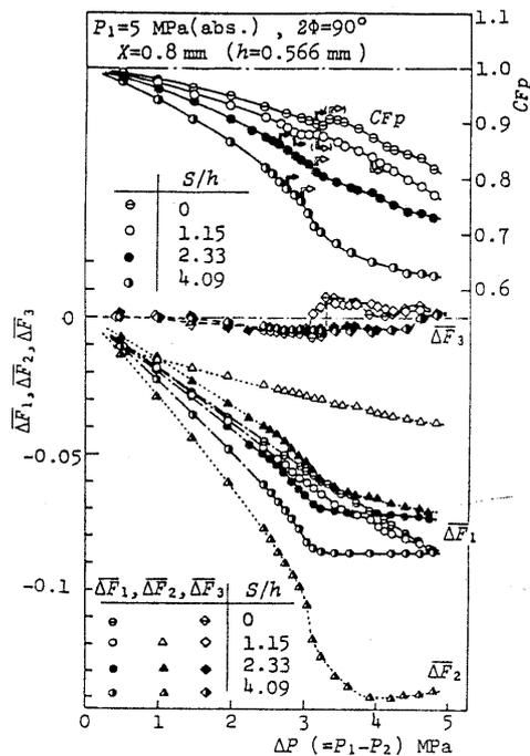
Fig.6 Influence of the chamfer length (Half cut model, Diverging flow)
