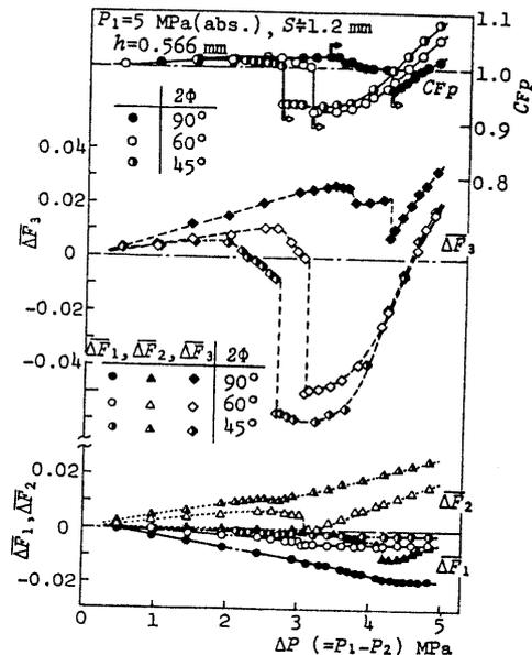
Fig.10 Influence of the poppet angle (Half cut model, Converging flow,  $S=1.2$  mm)
