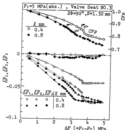
Fig.3 Influence of the valve lift (Half cut model, Diverging flow)
