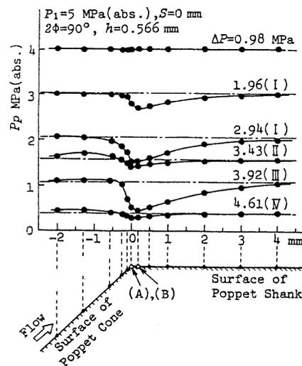
Fig.13 Alteration of the pressure distribution along the poppet surface in the downstream region (Diverging flow,  $2\phi=90^\circ$ ,  $S=0$  mm)
