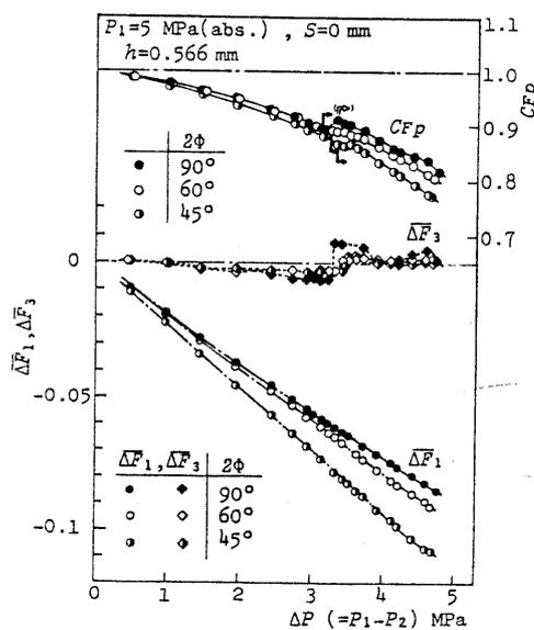
Fig.11 Influence of the poppet angle (Half cut model, Diverging flow,  $S=0$  mm)
