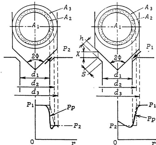
(a) Diverging flow (b) Converging flow
