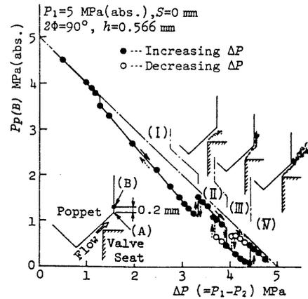
Fig.12 Alteration of the pressure at the point (B) (Diverging flow,  $2\phi=90^\circ$ ,  $S=0$  mm)
