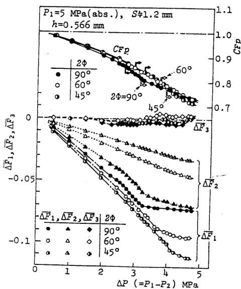
Fig.9 Influence of the poppet angle (Half cut model, Diverging flow,  $S=1.2$  mm)
