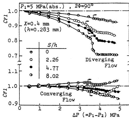
Fig.5 Influence of the chamfer length (Full shaped model)
