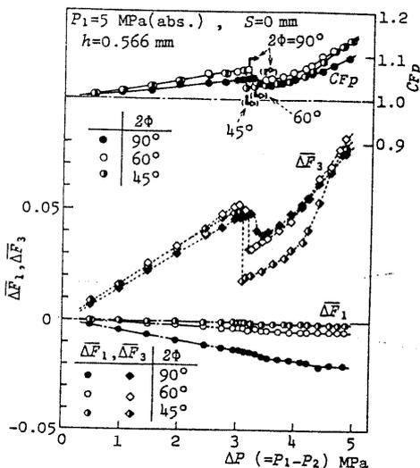
Fig. 14 Influence of the poppet angle (Half cut model, Converging flow,  $S=0$  mm)
