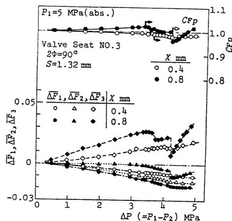
Fig.4 Influence of the valve lift (Half cut model, Converging flow)
