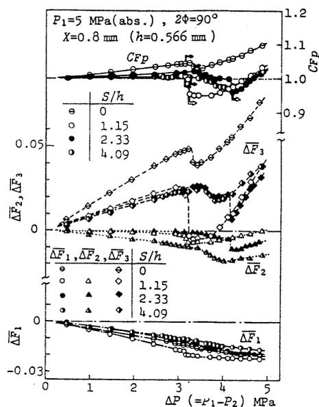
Fig.7 Influence of the chamfer length (Half cut model, Converging flow)
