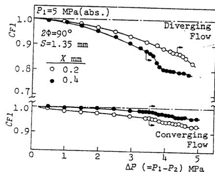
Fig.2 Influence of the valve lift (Full shaped model)
