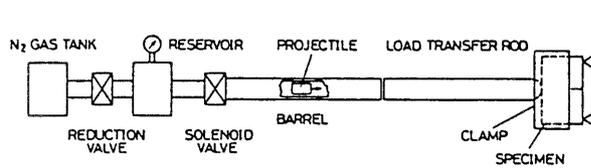
Fig. 2 Apparatus for impact loading
