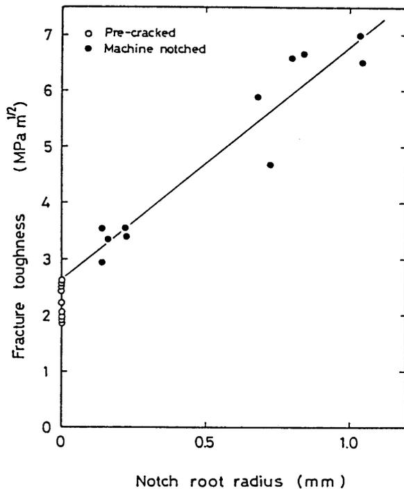
Fig. 8 Fracture toughness as a function of notch root radius
