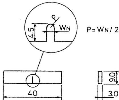
(b) Geometry and dimensions of notched specimen
