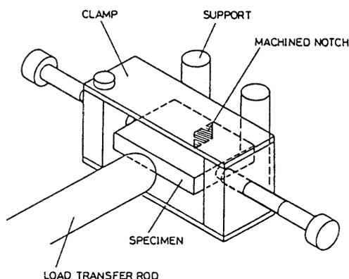
Fig. 3 Schematic view of clamp
