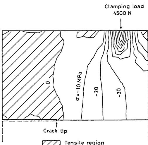
Fig. 4 Stress field in a specimen applied a clamping load
