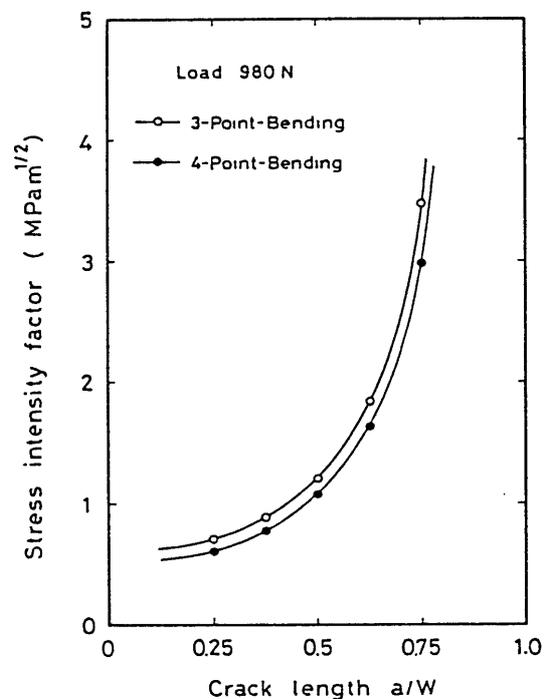
Fig. 5 Stress intensity factor-crack length curve for three-point and four-point bending specimens
