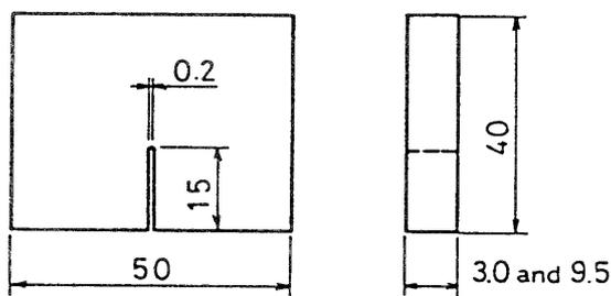
(a) Geometry and dimensions of pre-cracked specimen
