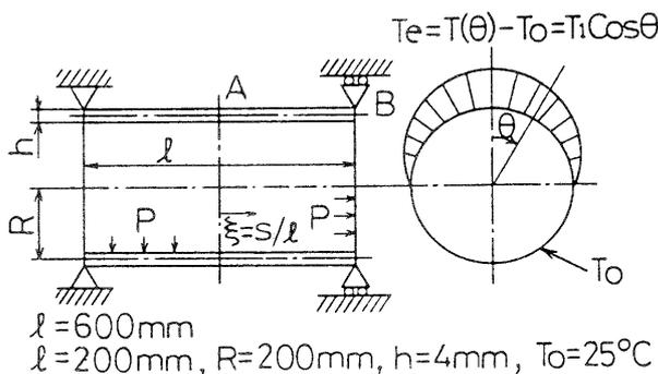
Fig. 2 Cylindrical shell and temperature distribution
