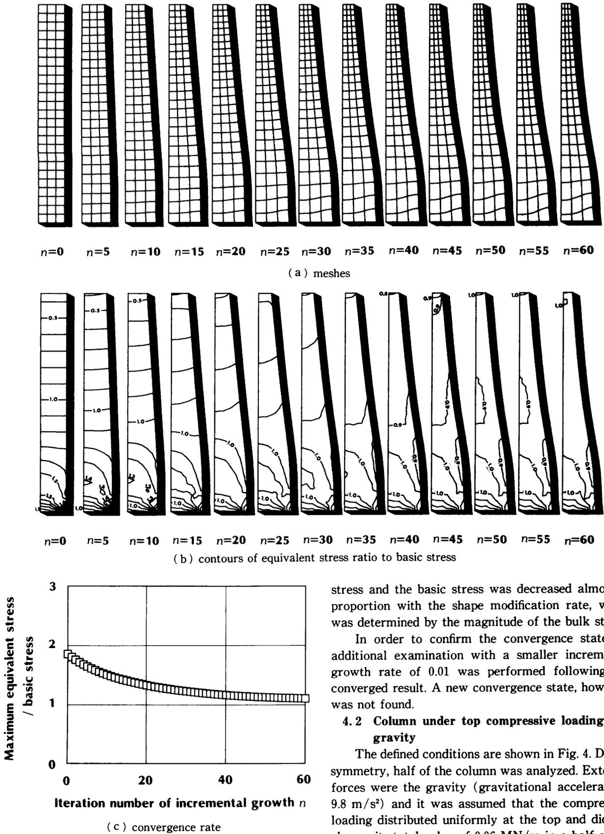
Fig. 5 Results of the shape-optimization process in the column problem.
