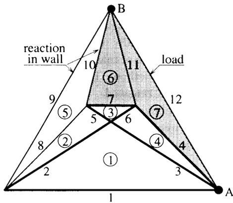
Fig. 2 Example of simplicial complex related to ground structure (a)
