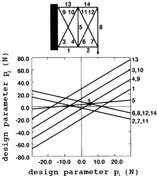
Fig. 5 Relation between design parameters  $p_1$  and  $p_2$
