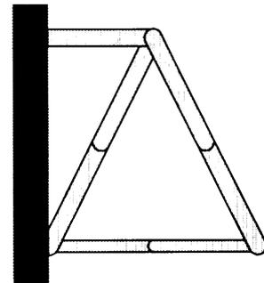
Fig. 6 Optimum structure obtained from ground structure (b)
