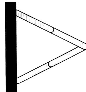
Fig. 7 Optimum structure obtained from ground structure (c)
