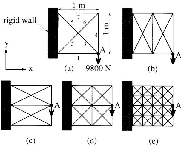
Fig. 1 Ground structures
