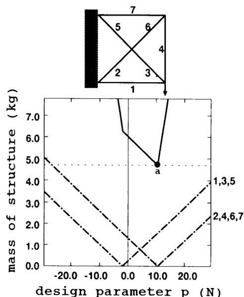
Fig. 3 Relation between design parameter and mass of structure
