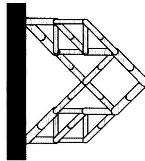
Fig. 12 Optimum structure obtained from ground structure (e) (II)
