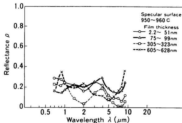
Fig. 4 Normal spectral reflectance of silicon wafers with oxide film
