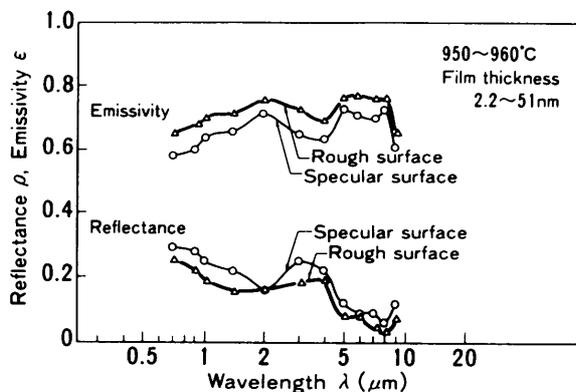
Fig. 8 Normal spectral emissivity and reflectance of specular surface and rough surface of silicon wafers with oxide film
