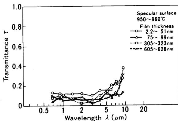
Fig. 5 Normal spectral transmittance of silicon wafers with oxide film
