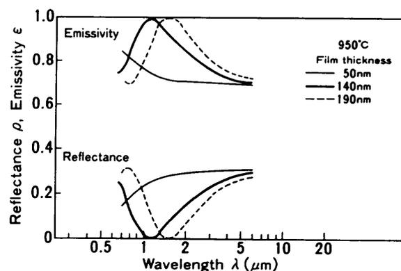
Fig. 10 Calculation results of emissivity and reflectance of silicon wafers with nitride film
