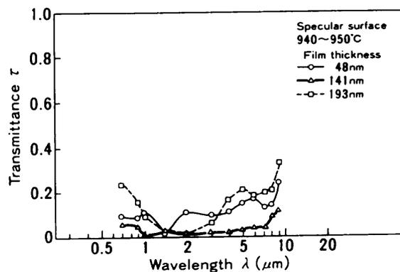
Fig. 7 Normal spectral transmittance of silicon wafers with nitride film
