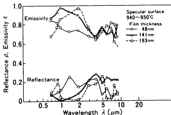
Fig. 6 Normal spectral emissivity and reflectance of silicon wafers with nitride film
