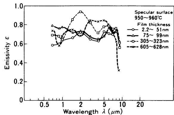
Fig. 3 Normal spectral emissivity of silicon wafers with oxide film
