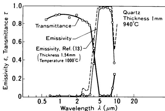
Fig. 2 Normal spectral emissivity and transmittance of quartz
