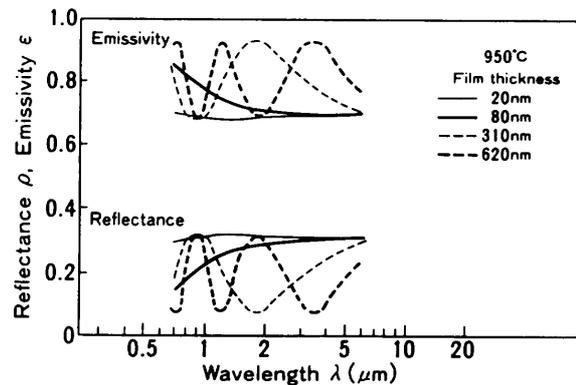
Fig. 9 Calculation results of emissivity and reflectance of silicon wafers with oxide film
