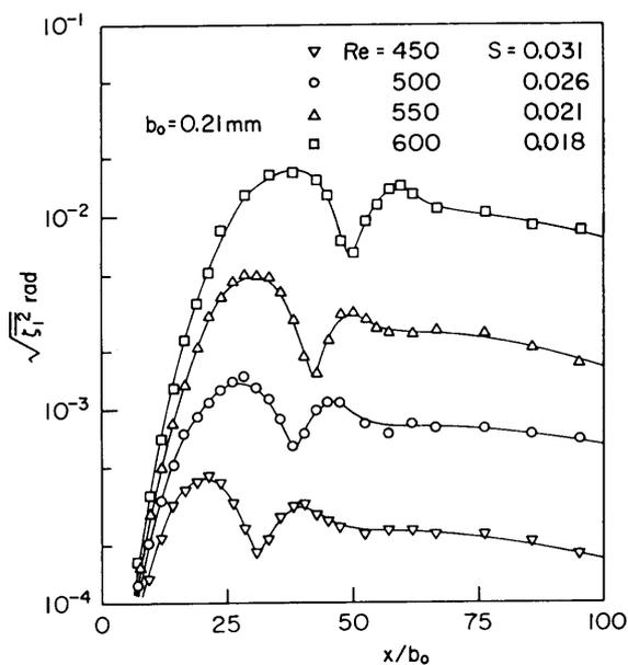
Fig. 6 Variation of root mean square of interfacial gradient with distance downstream from nozzle exit
