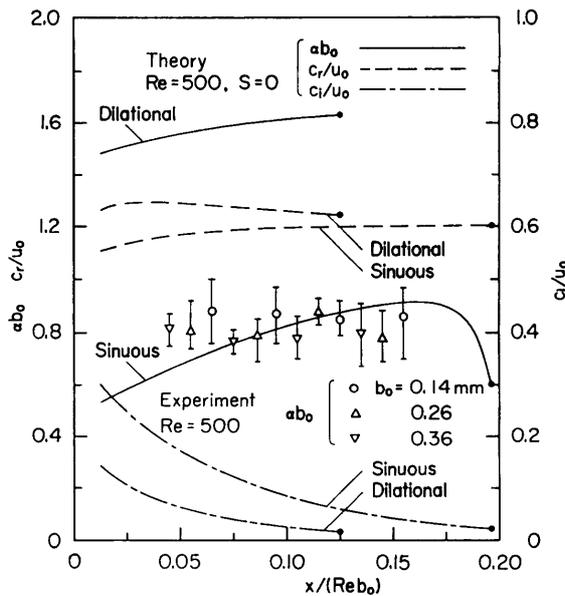
Fig. 8 Comparison of experimental results with numerical results on hard-mode instability
