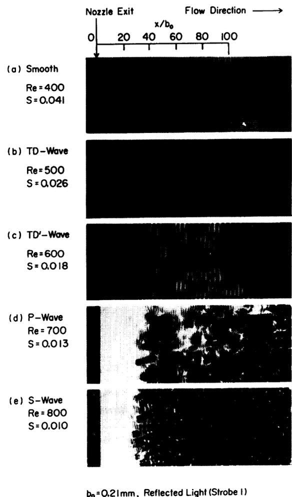
Fig. 3 Interfacial pattern of liquid sheet in stationary atmosphere
