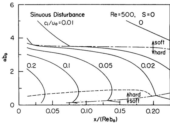
Fig. 7 Instability curves for sinuous disturbance
