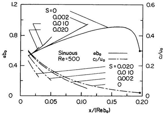
Fig. 10 Effect of  $S$  on hard-mode instability
