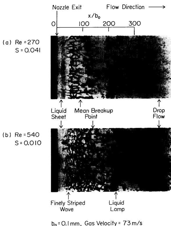
Fig. 1 Breakup patterns of liquid sheet in the gas stream
