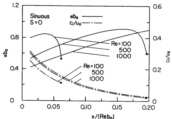
Fig. 9 Effect of  $Re$  on hard-mode instability
