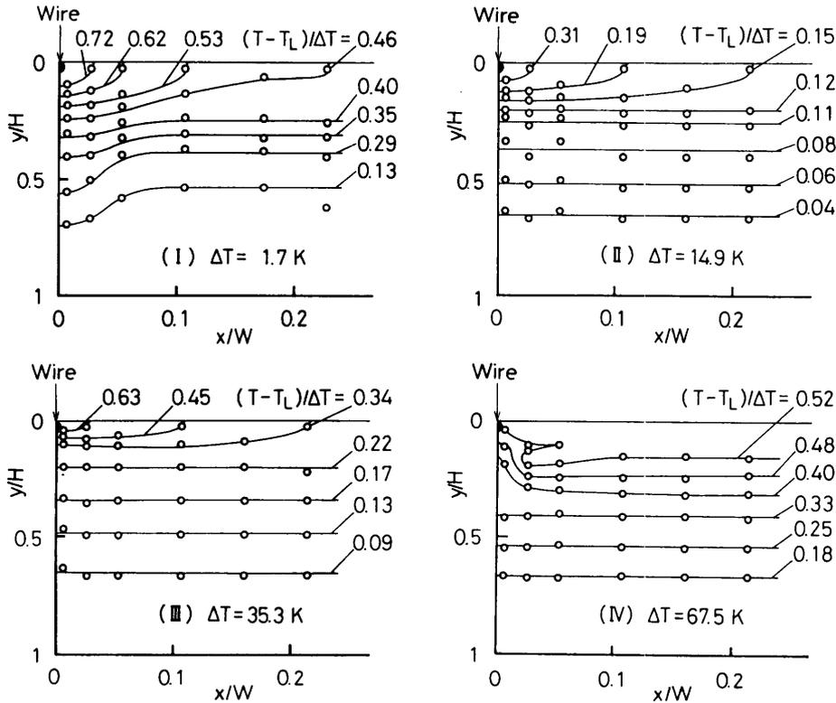
Fig. 7 Representative temperature distributions around wire ( $d=0.2$  mm,  $H=15$  mm, liquid: *n*-propanol)
