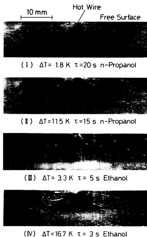
Fig. 6 Representative flow patterns around wire ( $d=0.2$  mm,  $H=15$  mm)
