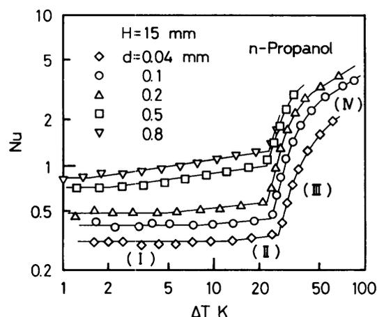
Fig. 4 Variations of Nusselt number of wire with temperature difference (effect of wire diameter)
