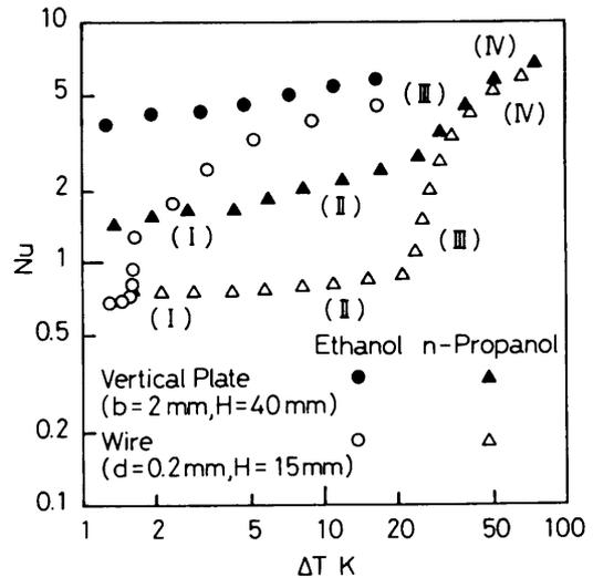
Fig. 11 Variations of Nusselt number of vertical plate with temperature difference
