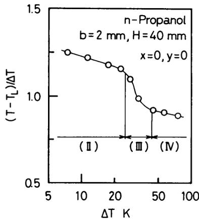
Fig. 14 Temperature of liquid surface in contact with top of plate
