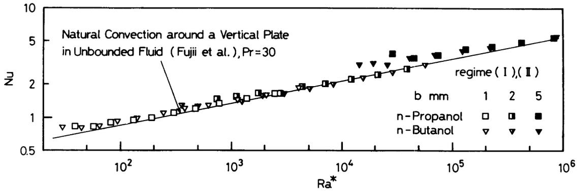
Fig. 12 Relationship between modified Rayleigh number and Nusselt number of vertical plate
