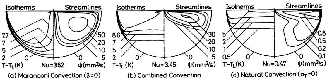
Fig. 2 Representative numerical results. ( $T_H - T_L = 50$  K,  $d = 0.2$  mm,  $W = 50$  mm, liquid: *n*-propanol (300 K))
