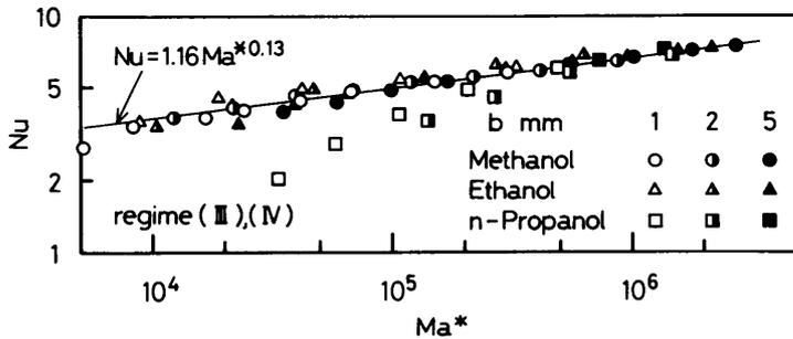
Fig. 13 Relationship between modified Marangoni number and Nusselt number of vertical plate
