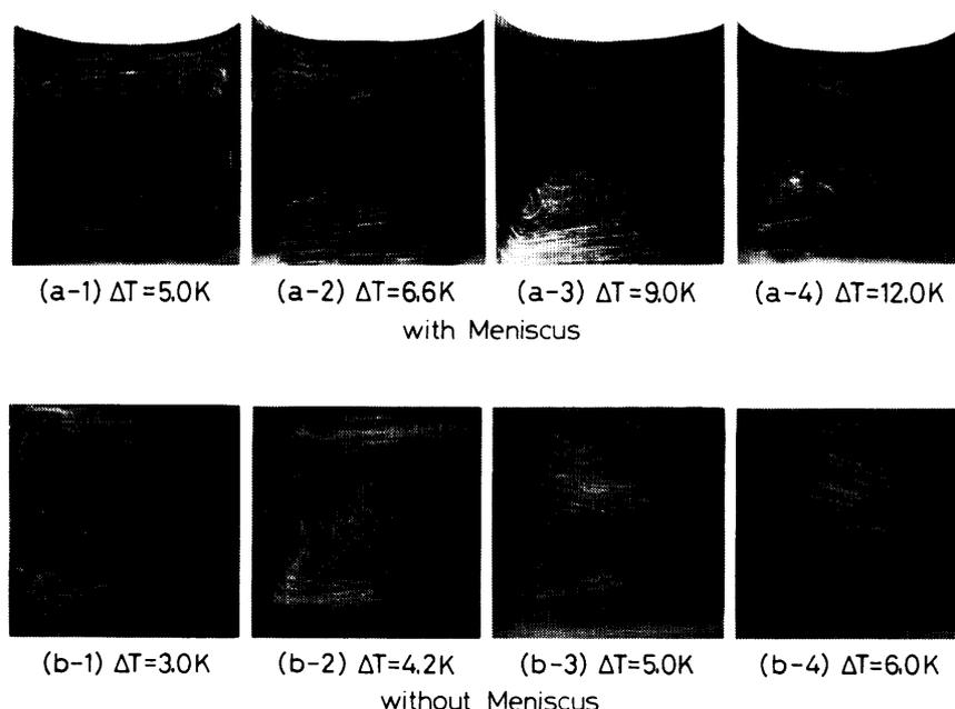
Fig. 16 Representative flow patterns in rectangular cavity heated from the side (liquid: ethanol + *n*-propanol (90 : 10 wt%))
