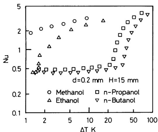
Fig. 5 Variations of Nusselt number of wire with temperature difference (effect of test liquid)
