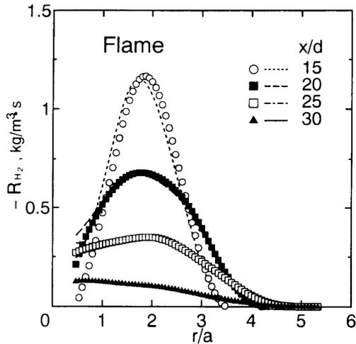
Fig. 4 Radial profiles of local reaction rate of  $H_2$  on the cross section. Symbols indicate axial position in  $x/d$ . They are demonstration as well as Figs. 3.
