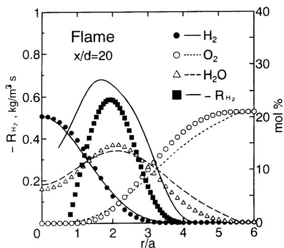
Fig. 7 Radial profiles of local reaction rate of  $H_2$  and concentrations of  $H_2$ ,  $O_2$ , and  $H_2O$  on the cross section of  $x/d=20$ . Plot is conducted with the experimental data by using Method A and line shows the simulation results.
