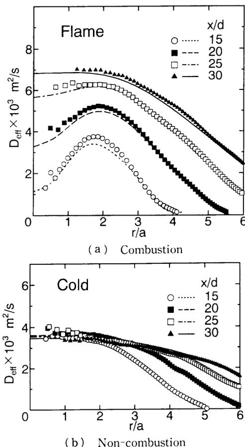
Fig. 3 Radial profiles of effective diffusion coefficient on the cross section. Symbols indicate axial position in  $x/d$ . They are demonstration to examine the accuracy of calculation program. Plot and line are obtained from Method A and Method B, respectively.
