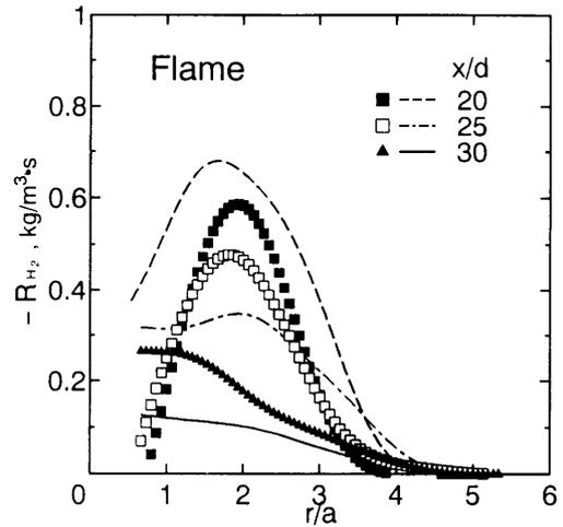
Fig. 6 Radial profiles of local reaction rate of  $H_2$  on the cross section. Symbols indicate axial position in  $x/d$ . Plot is conducted with the experimental data by using Method A and line shows the simulation results.
