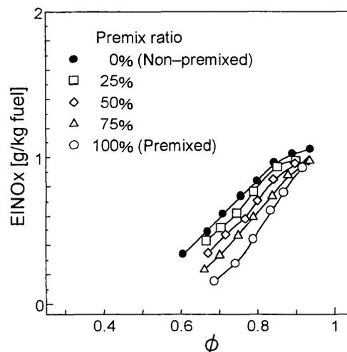
Fig. 8  $\text{NO}_x$  emission in partially premixed combustion,  $Q_{ma}=183$  l/min,  $\phi=0.7$
