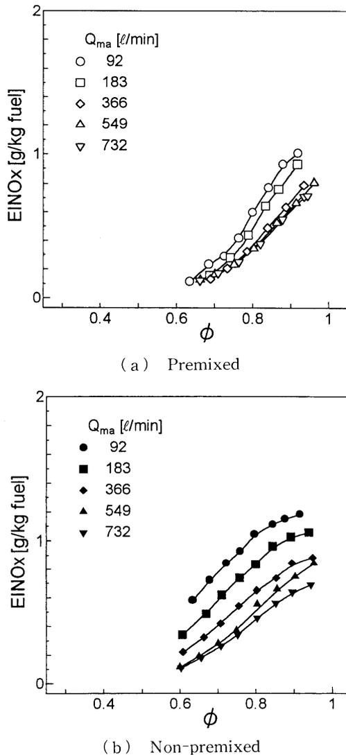
Fig. 4 NO<sub>x</sub> emission in premixed and non-premixed combustion
