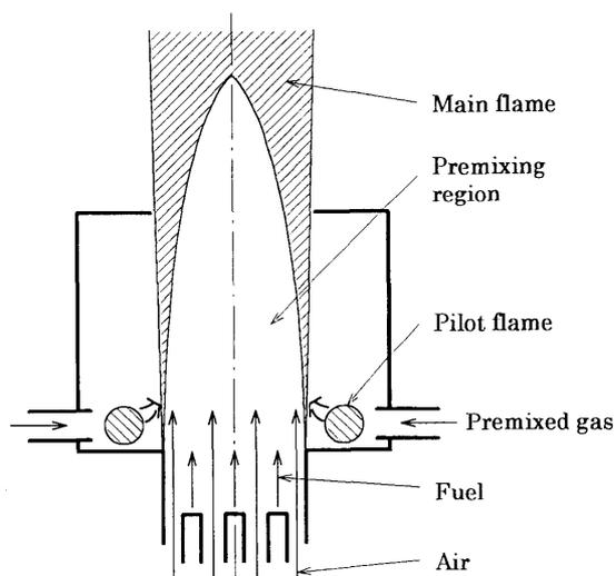
Fig. 7 Combustion mechanism of cyclone-jet combustor
