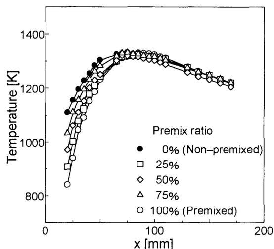
Fig. 9 Comparison of axial temperature distributions for partially premixed flames,  $Q_{ma}=183$  l/min,  $\phi=0.7$
