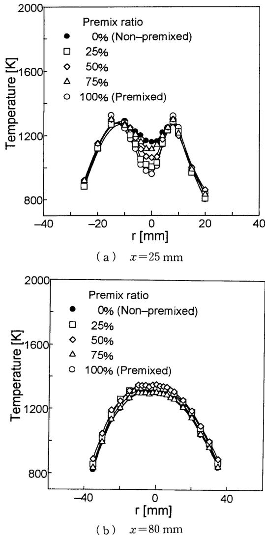
Fig. 10 Comparison of radial temperature distributions for partially premixed flames,  $Q_{ma}=1831/\text{min}$ ,  $\phi=0.7$
