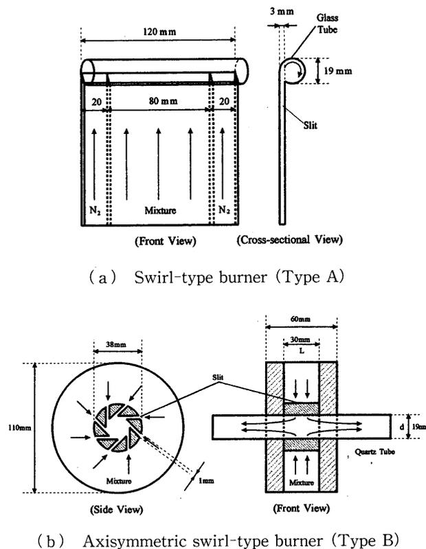
Fig. 1 Swirl-type burners used in this study
