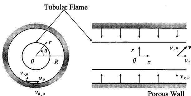
Fig. 2 Axially symmetric flow field in an infinitely long rotating porous tube with uniform injection
