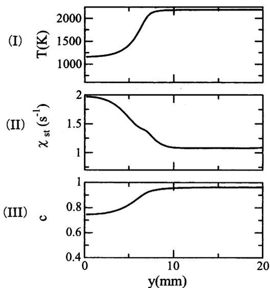
Fig. 5 (I) Temperature, (II) scalar dissipation rate, and (III) progress variable for stoichiometric line of case 2
