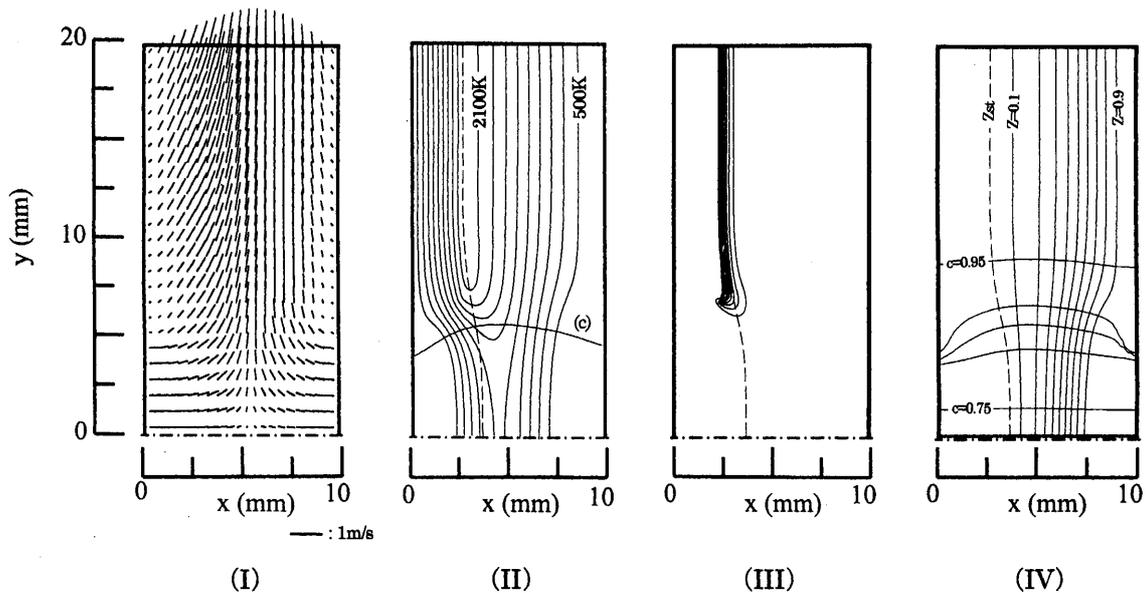
Fig. 4 Calculated flow and scalar fields for case 2: (I) Velocity vectors, (II) temperature, (III) heat-release rate (30–300 MJ/m<sup>3</sup> s), and (IV) distribution of mixture fraction and progress variable
