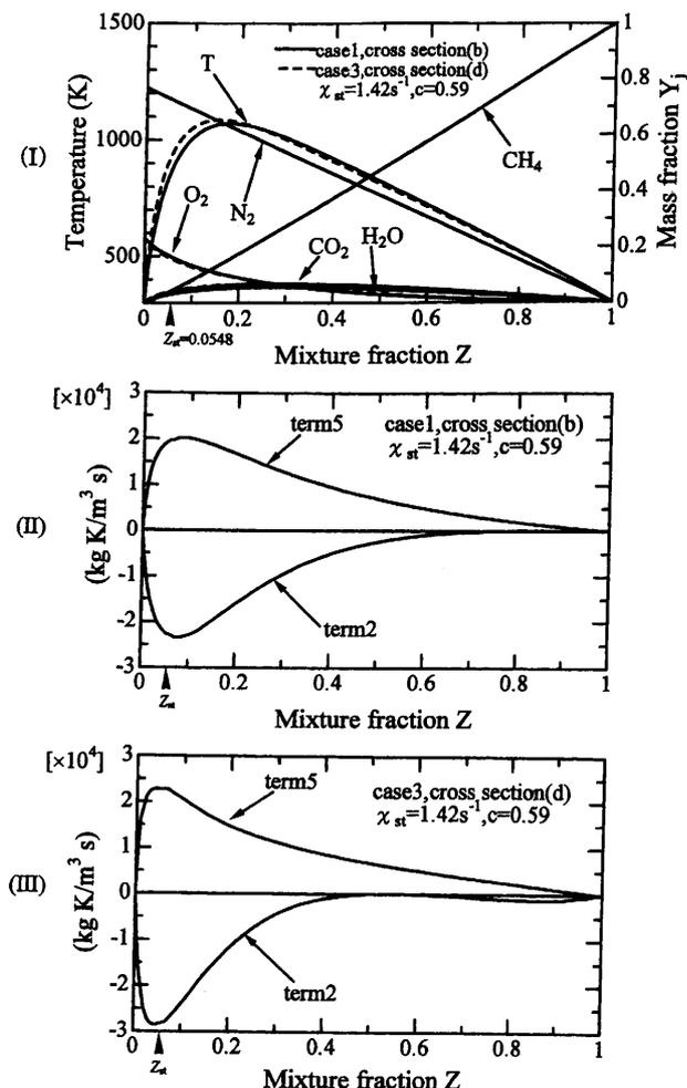
Fig. 10 (I) Comparison of flame structures between cross-section (b) of case 1 (Fig. 2) and cross-section (d) of case 3 (not shown). (II) Heat transfer balance for cross-section (b). (III) Heat transfer balance for cross-section (d). Conditions are  $\chi_{st} = 1.42 \text{ s}^{-1}$  and  $c = 0.59$ .
