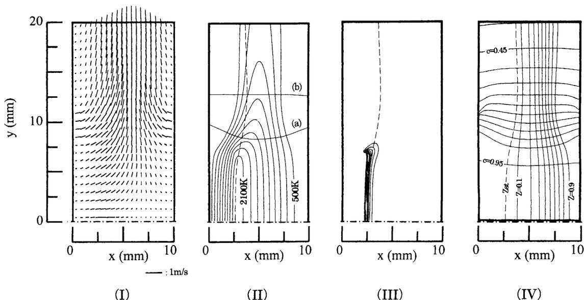
Fig. 2 Calculated flow and scalar fields for case 1: (I) Velocity vectors, (II) temperature, (III) heat-release rate ( $30 - 300 \text{ MJ/m}^3\text{s}$ ), and (IV) distribution of mixture fraction and progress variable
