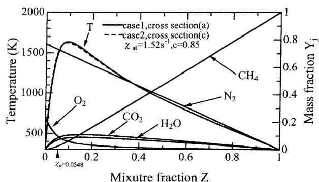
Fig. 9 Comparison of flame structures between cross-section (a) of case 1 and cross-section (c) of case 2 for the condition of  $\chi_{st} = 1.52 \text{ s}^{-1}$  and  $c = 0.85$
