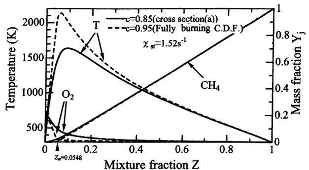
Fig. 7 Comparison of flame structures between fully burning counterflow nonpremixed flame without extinction and cross-section (a) of case 1 (Fig. 2) for the same scalar dissipation rate ( $\chi_{st} = 1.52 \text{ s}^{-1}$ ). CDF: counterflow diffusion flame (nonpremixed)
