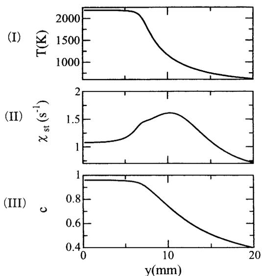
Fig. 3 (I) Temperature, (II) scalar dissipation rate, and (III) progress variable for stoichiometric line of case 1
