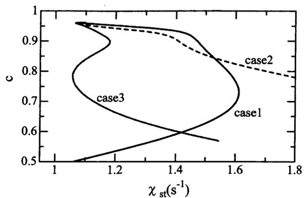
Fig. 6 Progress variable for each case as a function of scalar dissipation rate
