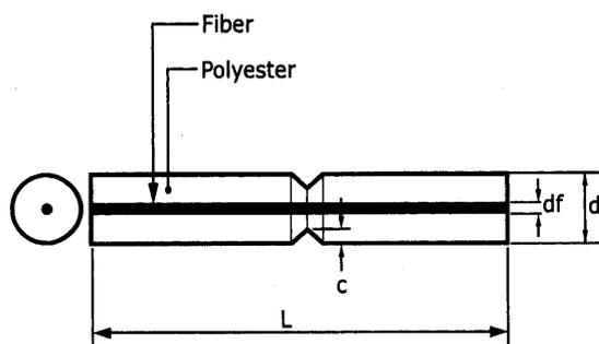
Fig. 1 Specimen geometry and dimension
