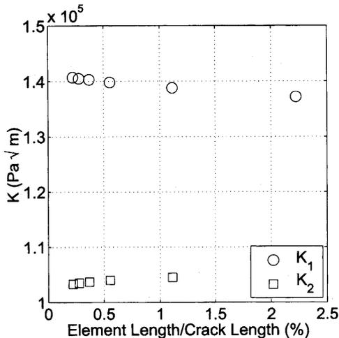
Fig. 20 Sensitivity of stress intensity factor to mesh size
