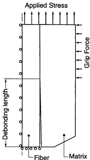
Fig. 8 Boundary condition in finite element model
