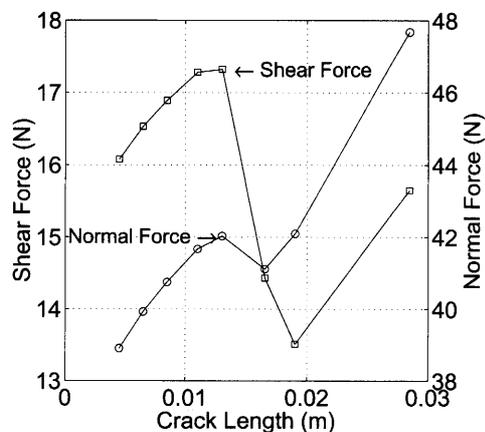
Fig. 11 Spring forces in normal and shear directions for various crack length
