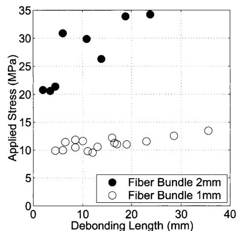
Fig. 6 Debonding length versus applied stress
