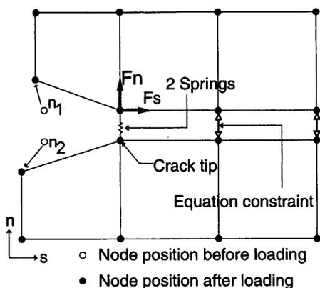
Fig. 7 Interface spring model
