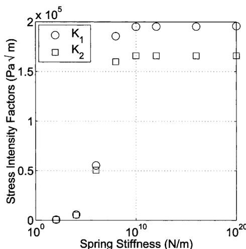
Fig. 19 Sensitivity of stress intensity factors to springs stiffness
