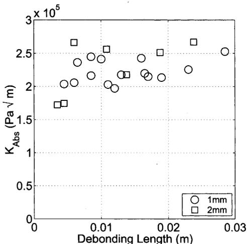
Fig. 16 Absolute stress intensity factor versus debonding length
