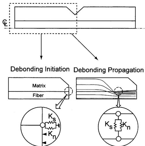
Fig. 9 Specimen model and implementation of springs to the crack tip
