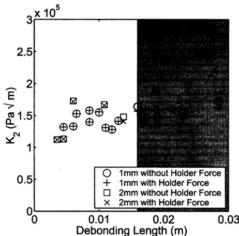
Fig. 15 Shearing mode stress intensity factor versus debonding length
