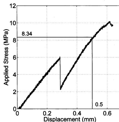
Fig. 3 Typical load-displacement diagram applied nominal stress versus deflection.
