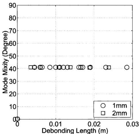
Fig. 17 Mode mixity  $\psi$  versus debonding length
