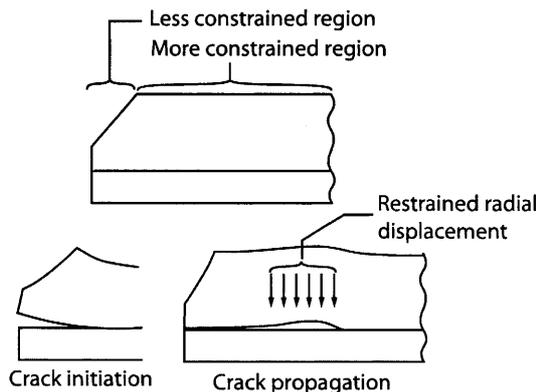
Fig. 18 Restrained radial displacement when crack propagated
