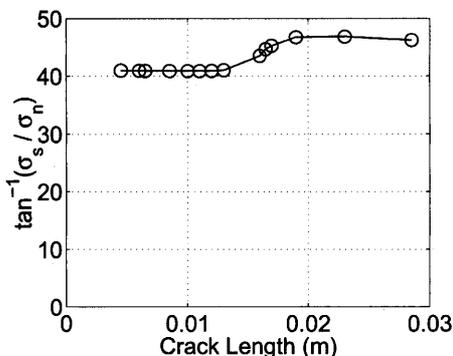
Fig. 13 Ratio of normal and shear stresses at near the crack tip
