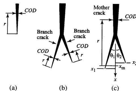
Fig. 4 Measurement of crack opening displacement
