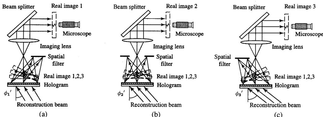
Fig. 3 Reconstruction and microscopic photographing of crack images
