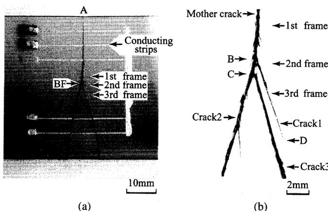
Fig. 6 (a) Specimen after fracture (b) Enlarged picture around the bifurcation point
