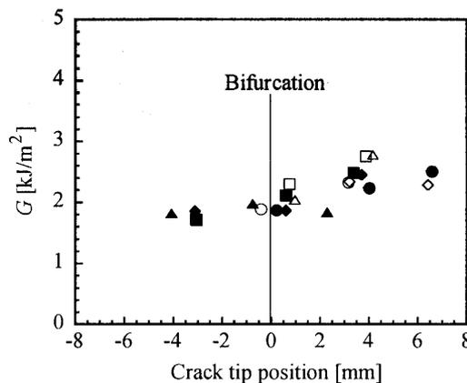
Fig. 10 Energy release rate near the bifurcation point
