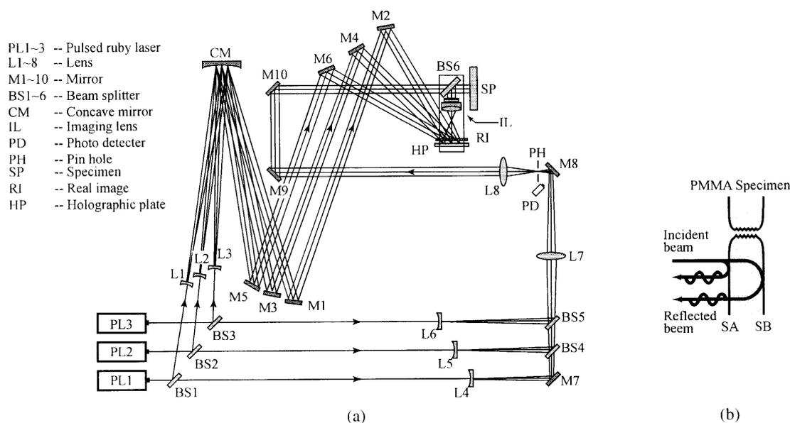
Fig. 2 Holographic recording system for rapidly bifurcating cracks
