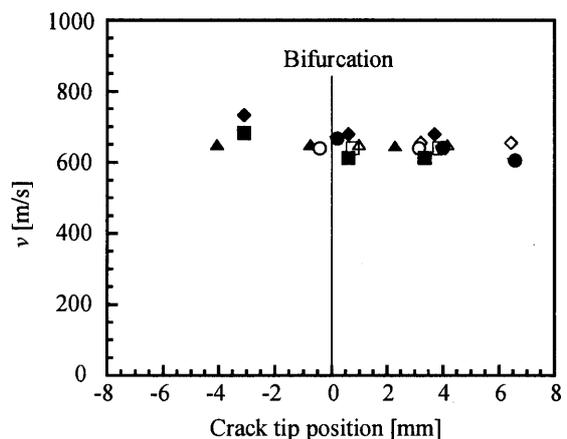
Fig. 9 Crack speed near the bifurcation point
