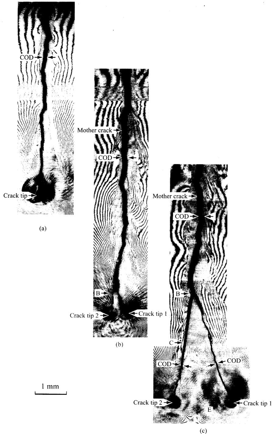
Fig. 7 Microscopic photographs of rapidly bifurcating crack
