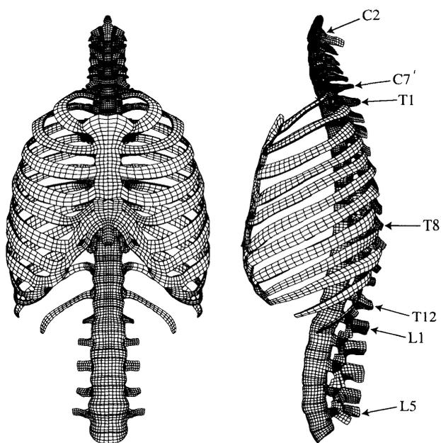
Fig. 1 Finite element model with thoracic cage
