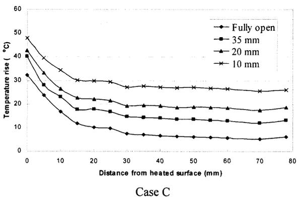
Figure 3 Outgoing temperatures distributions across the cavity gap tilted at 30° and a heat production of 150 W/m<sup>2</sup>
