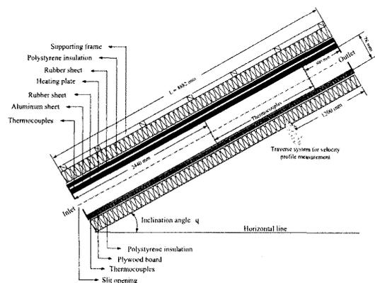
(b) Sectional diagram of cavity model
