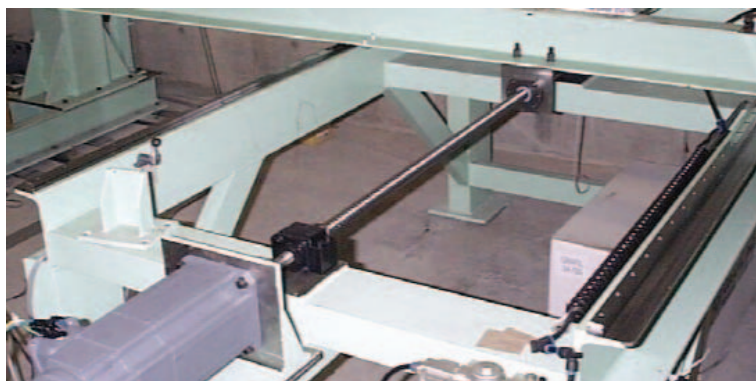
Fig. 2.7 Photograph of actuation mechanism for Traverse unit
