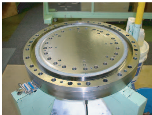
Fig. 6.1 Photograph of Ring burst test machine for CFRP ring
