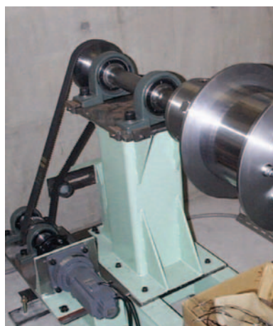
Fig. 2.6 Photograph of actuation mechanism for Mandrel unit
