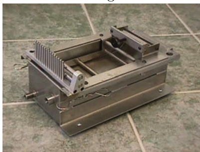
(b) Resin-bath without coating roll
