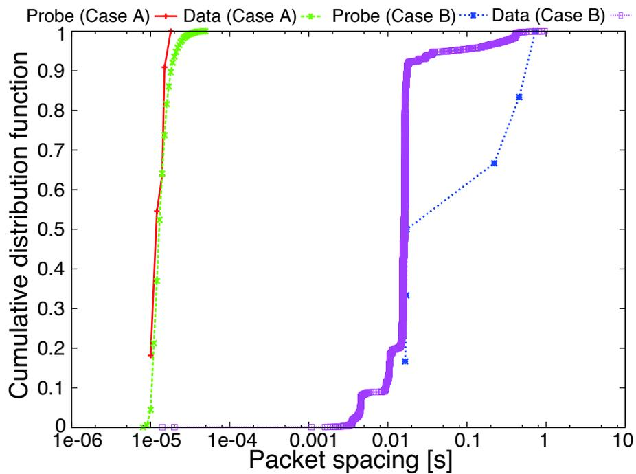
FIGURE 4.3: CDF of packet spacing for connection pair at cases A and B.
