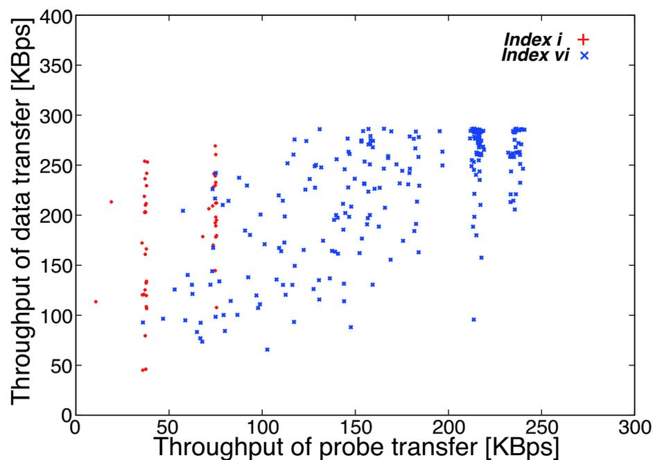
FIGURE 2.18: Connection pair throughput at indices  $i$  and  $vi$ .
