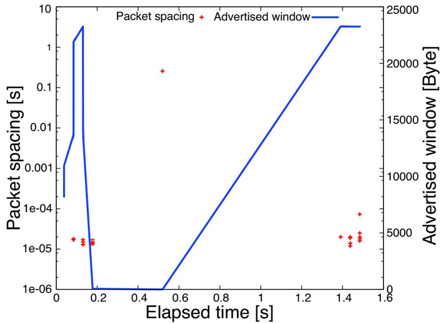
(a) Packet spacing and advertised window of probe transfer at  $\beta$  (64KB)
