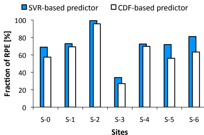
FIGURE 6.5: Fraction of RPE within 10% or less.
