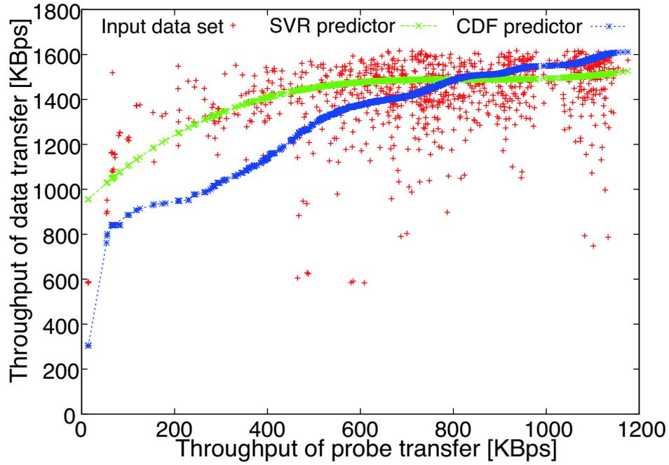
FIGURE 5.7: Prediction results at node pair  $(\eta, \theta)$ .
