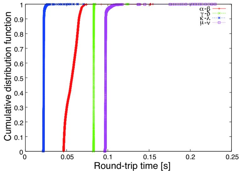
FIGURE 2.6: CDF of RTT of data transfer at all node pairs (32MB).
