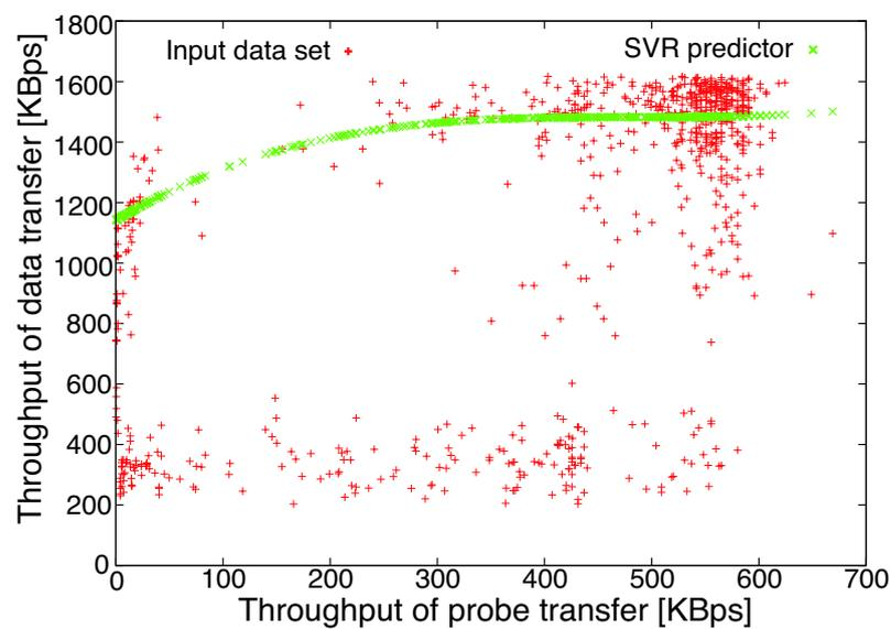
FIGURE 5.16: Prediction results at node pair  $(\eta, \theta)$ .
