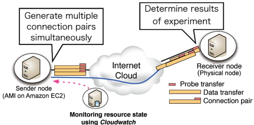
FIGURE 2.17: Throughput measurement method on Amazon EC2.
