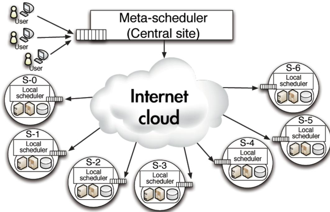
FIGURE 6.7: Simulation model.
