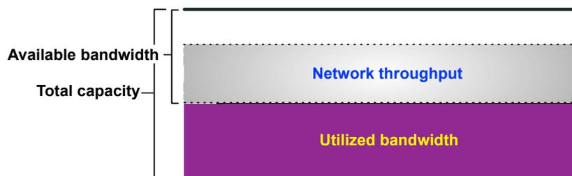
FIGURE 1.3: Composition of bandwidth on end nodes.
