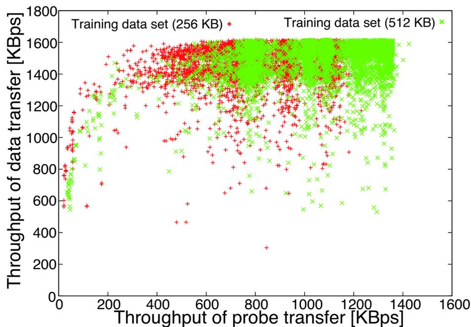
FIGURE 5.11: Actual throughput of training data sets at node pair  $(\eta, \theta)$ .
