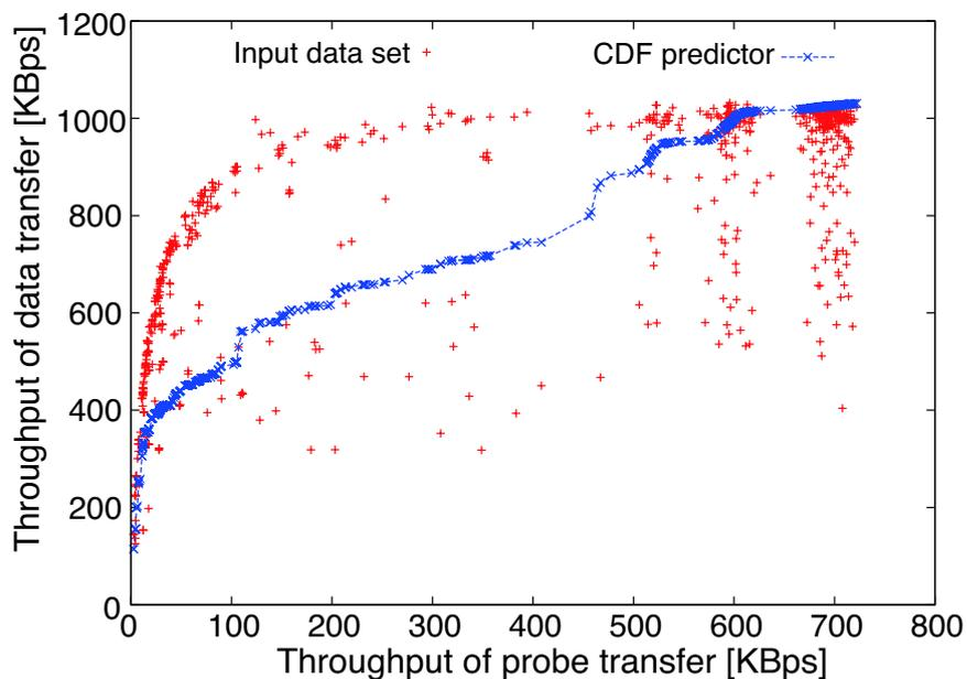
FIGURE 5.4: Prediction results of CDF-based predictor at node pair  $(\kappa, \lambda)$ .
