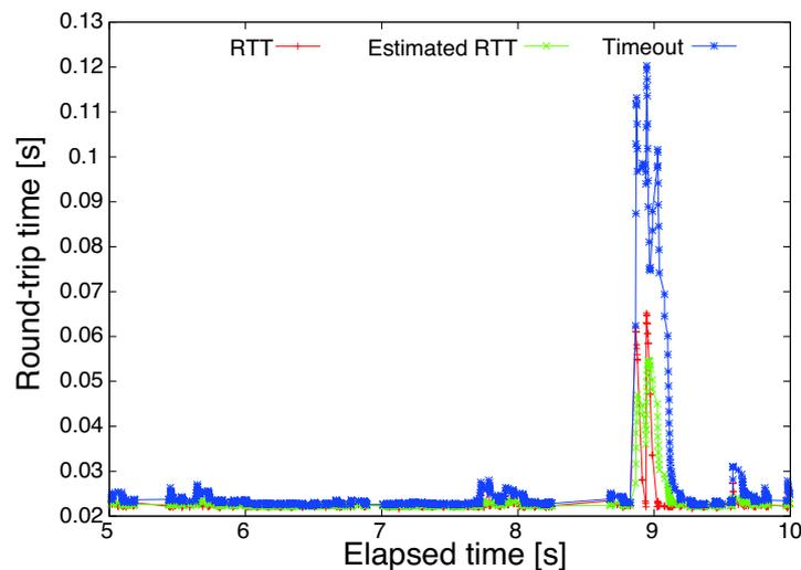
FIGURE 2.7: RTT, Estimated RTT, and Timeout of data transfer at pair  $(\kappa, \lambda)$ .
