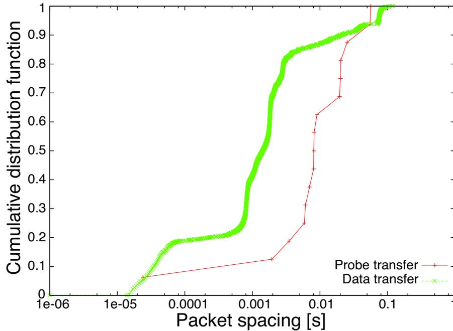
FIGURE 3.3: CDF of packet spacing at node  $\delta$ .
