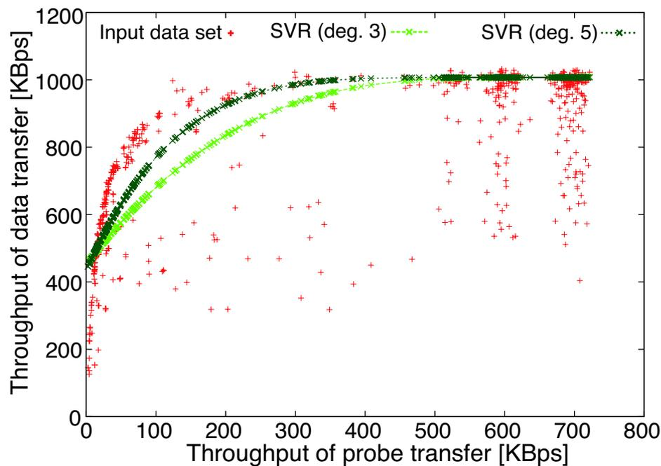
FIGURE 5.10: Prediction results with degree 3 and 5 at node pair  $(\kappa, \lambda)$ .
