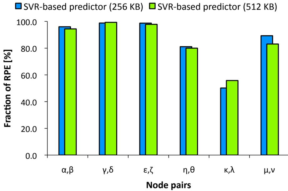
FIGURE 5.13: Fraction of RPE within 10% or less with 512-KB probes.
