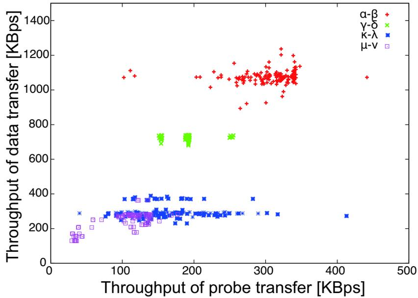
FIGURE 2.5: Throughput measurement results (probe: 64 KB, data : 32 MB).
