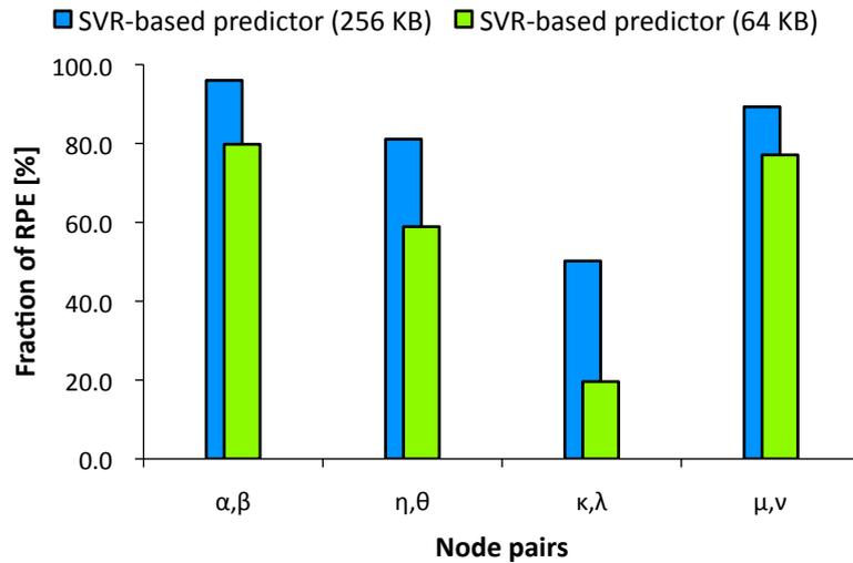
FIGURE 5.17: Fraction of RPE within 10% or less with 64-KB probes.
