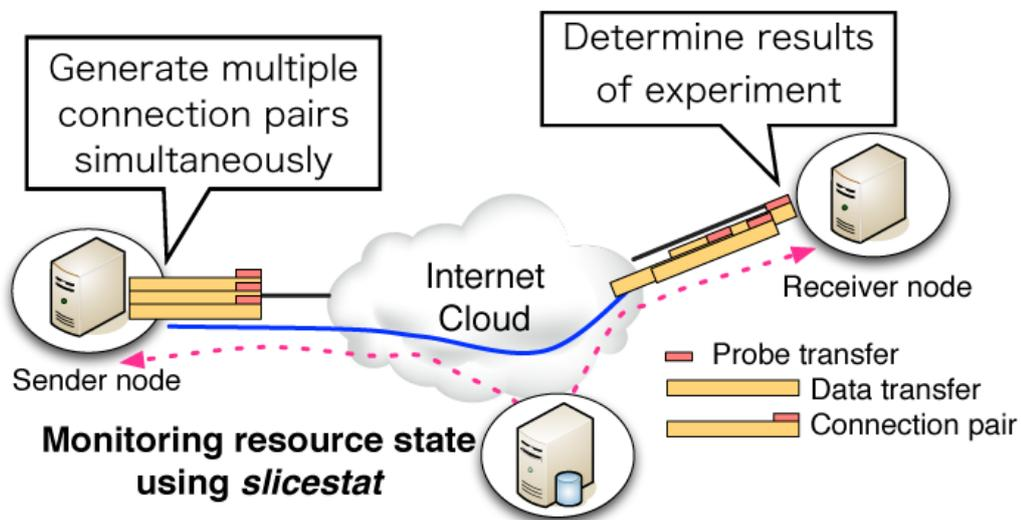
FIGURE 2.4: Connection pair measurement method with resource monitoring.
