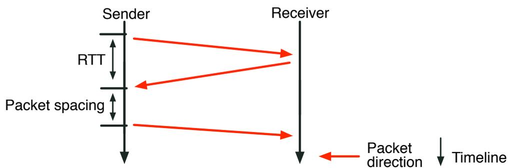
FIGURE 2.1: Concept of packet spacing.
