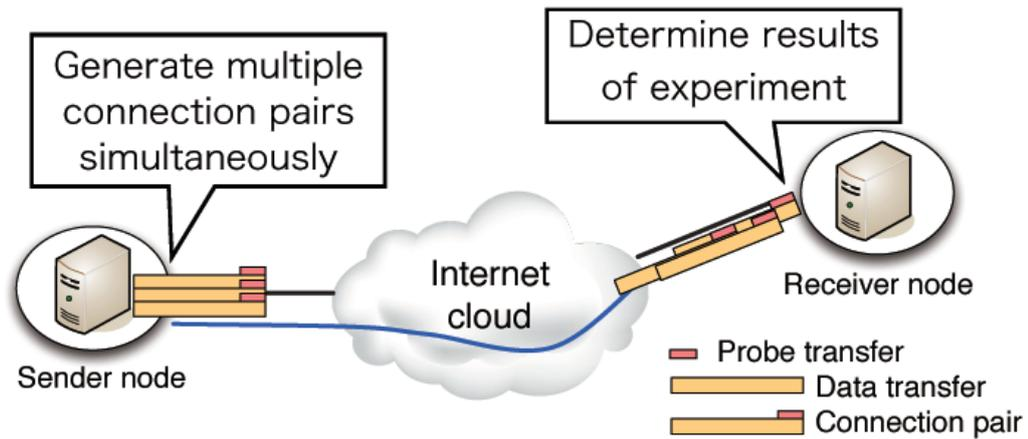
FIGURE 4.1: Measurement methodology.
