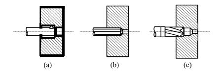
Fig. 5-2 (a) boring enlarges a hole; (b) reaming produces a slightly enlarged a hole that has a more accurate diameter; (c) counterboring enlarges a part of the hole so that the bottom part of the enlarged portion of the hole is flat and square
