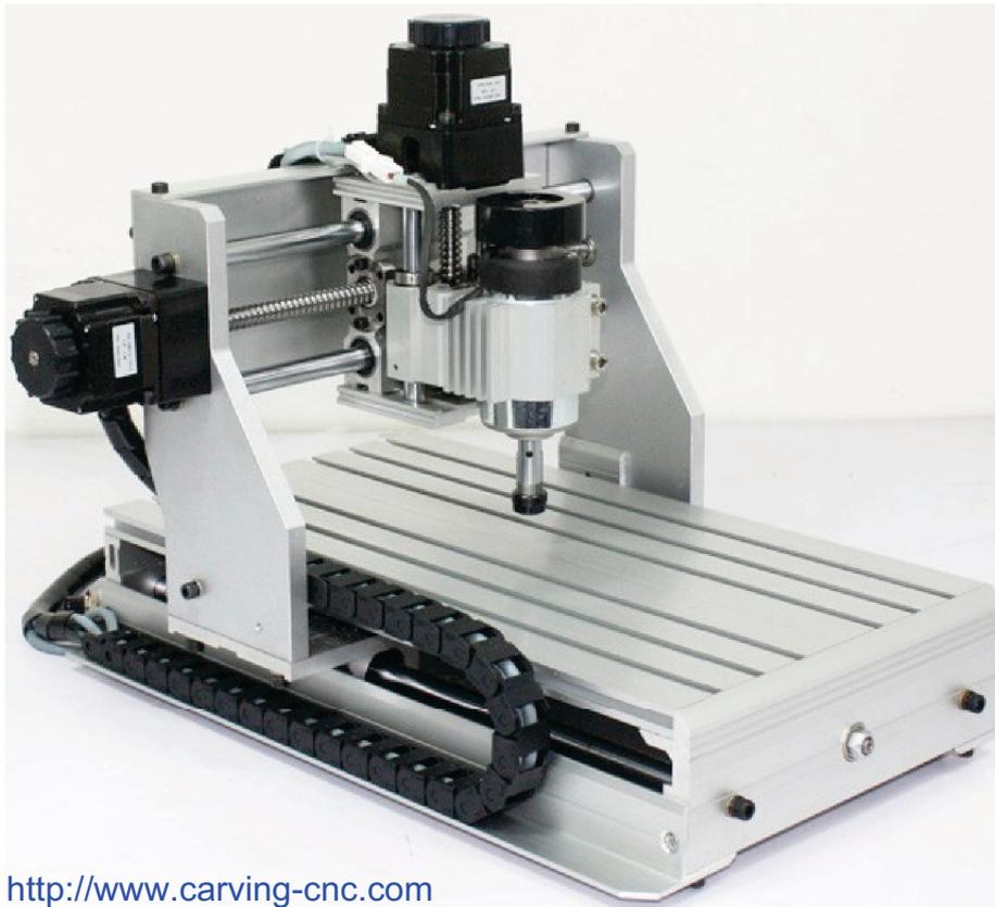
FIGURE 1.1: Application of ball screw feed drive in CNC machines
