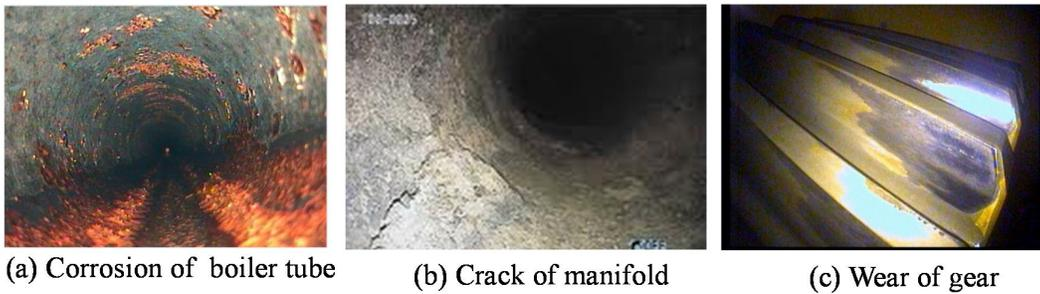
Fig 1.4. Applications of borescope in engineering field.
