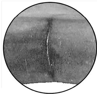
(b) Crack due to delay fracture
