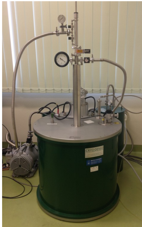
Figure 5. 26 Cryogenic liquid helium cryostat from 1.6 to 300K.
