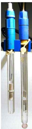
Figure 1.2 Ag/AgCl reference electrode (left) and glass electrode (right).
