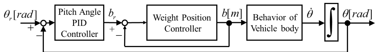
Fig. A.5 Block diagram of attitude control system of vehicle body
