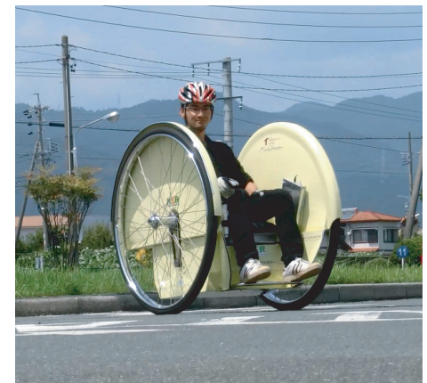
Fig. 2.1 Proposed parallel two-wheel vehicle with lower gravity center of vehicle body
