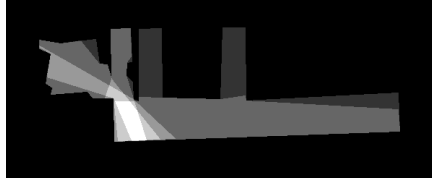
Figure 3.4: Face cost map of the arrangement in Fig. 3.3. Brighter face means it is seen by more guards.
