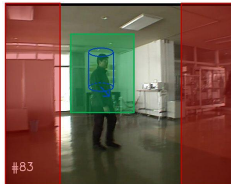
Figure 6.5: Region of Interest (ROI) for tracking. The red transparent shadows are places which has a high probability that person may appear to the scene from the side. The green transparent shadow is the ROI of the tracker. The blue cylinder denotes the current tracker bounding box.
