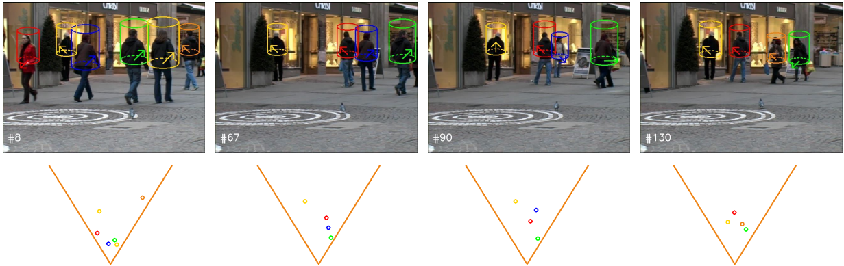
Figure 6.10: Human upper body orientation estimation results on TUD-Stadtmitte datasets using our proposed framework. Top sequence shows the detection (bounding boxes) and orientation estimation (arrows) results. Bottom sequence shows the estimated position of each detected person (circles) in the 3D world coordinate, with respect to the person position in the top images. Two orange line segments in the bottom sequences denote the camera FOV.
