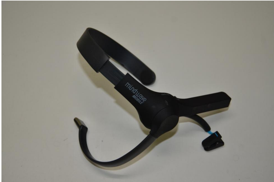
Figure 29. Mindwave EEG sensor
