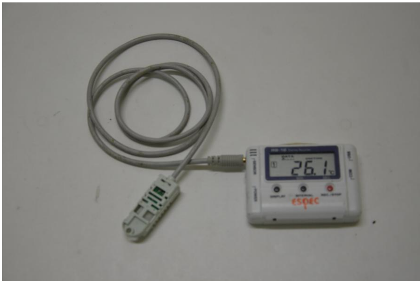
Figure 8. Espec RS-212 for air temperature monitoring
