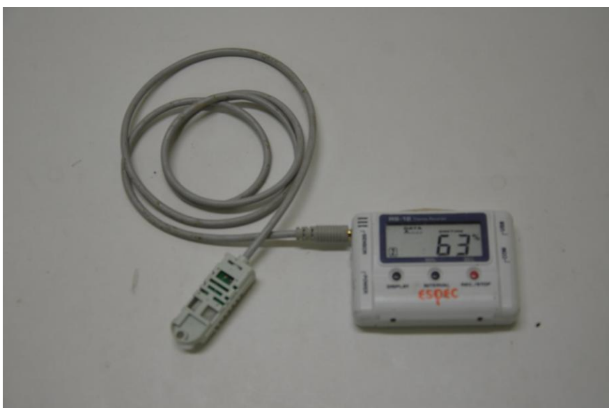
Figure 9. Espec RS-212 for air humidity monitoring
