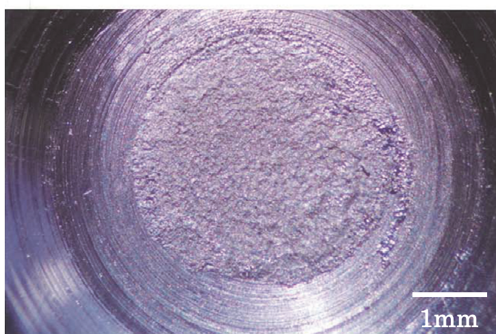
Fig. 3.9 Indentation surface of material A, 28kA-6cycles, no appearance of crack.
