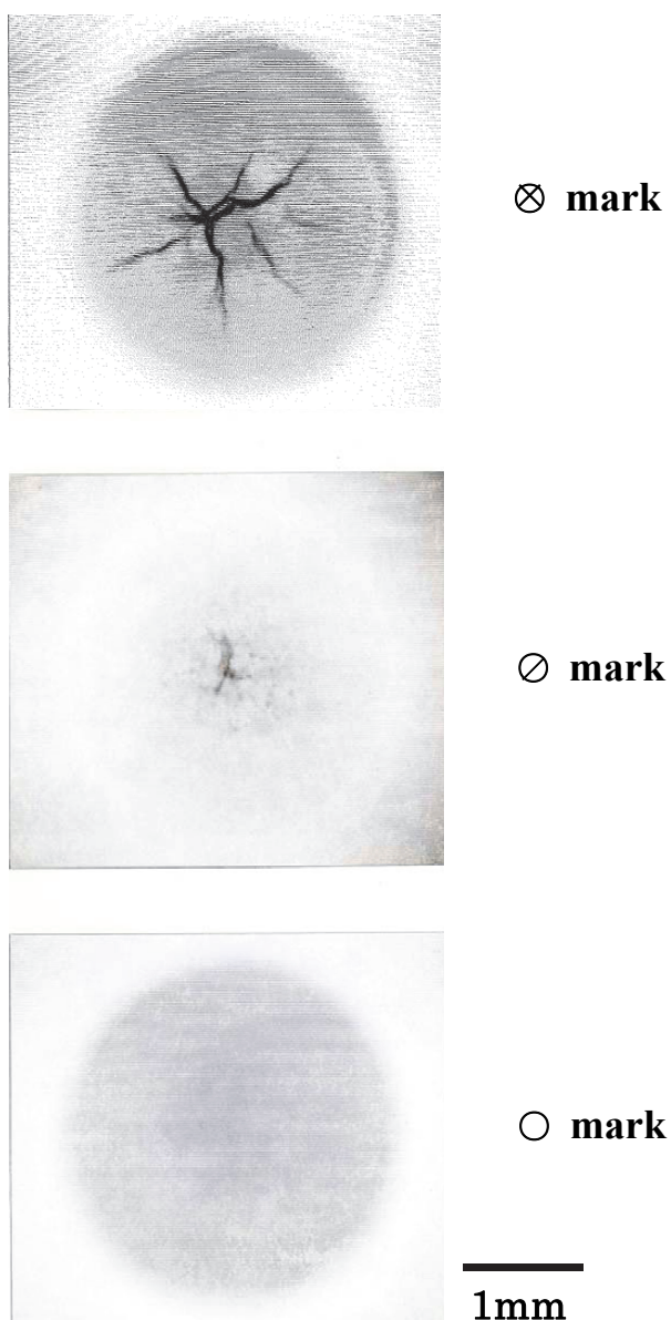
Fig. 3.16 Examples of classification of cracking.
