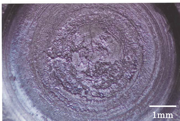
Fig. 3.3 Indentation surface of material A, 28kA-6cycles (No.1), appearance of center crack.
