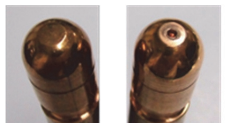
Fig. 2.3 Form of electrode tip.
