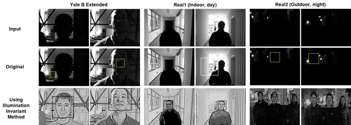
Figure 4.16: Comparison of the performance of face detection without and with the illumination invariant method. Upper images show the input images. Middle images show the face detection results without illumination invariant method. Lower images show the face detection results with illumination invariant method. The first and the second column, the third and the fourth column, and the fifth and the sixth column show the results using "Yale B Extended" face database, "Real1" video dataset, and "Real2" video dataset, respectively.
