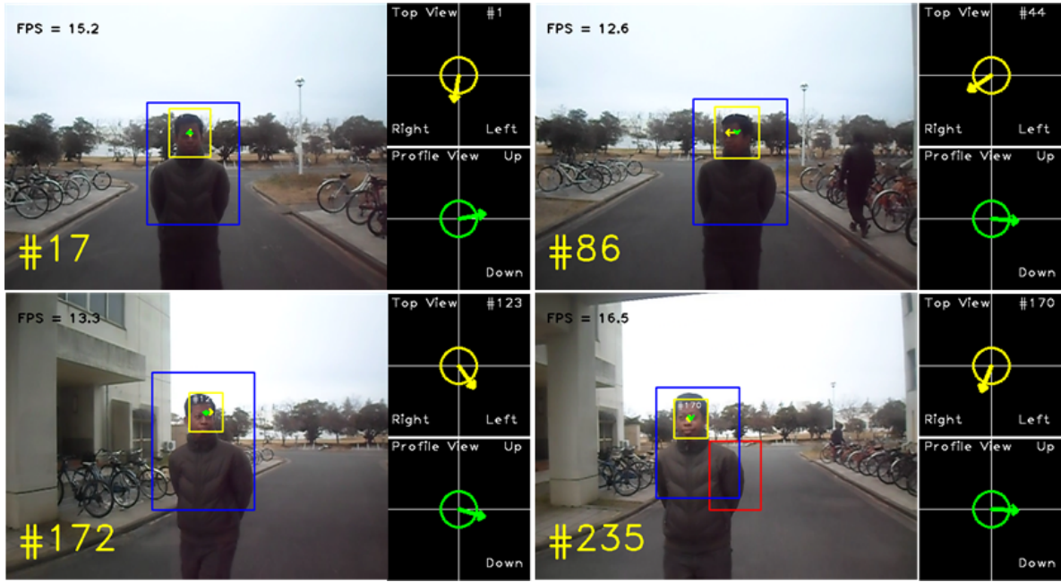
Figure 5.15: Experimental results of an online outdoor scene. First, the human upper body is detected and tracked (blue bounding box). Head detection and head orientation estimation supported by tracking is performed within the body's bounding box. The estimated head orientation is shown by yellow (pan) and green (tilt) arrows within the bounding box. The human upper body detection, the head detection and the head orientation estimation achieve good performances in this experiment.
