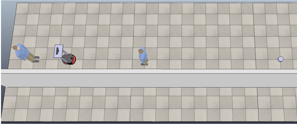
Figure 6.7: The situation that should be done by the robot in order to compare the performance of three QL-SFGM schemes: (1) QL-SFGM, (2) QL-SFGM + fixed PID, and (3) QL-SFGM + optimized PID. The wall is used to ascertain the robot take the same avoidance direction so that the trajectory can be compared visually.
