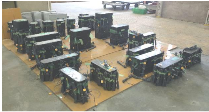
Figure 4-29 Specimens with and without strain gauges
