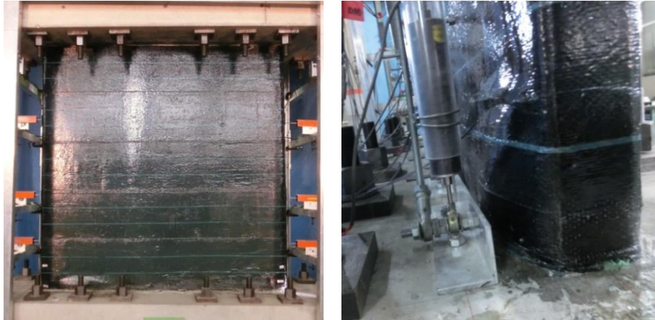
Figure 4-11 Failure of specimen RWF1
