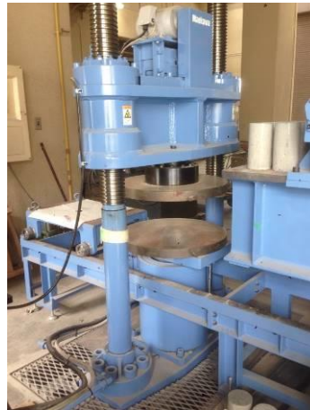
Figure 4-27 Compression loading machine
