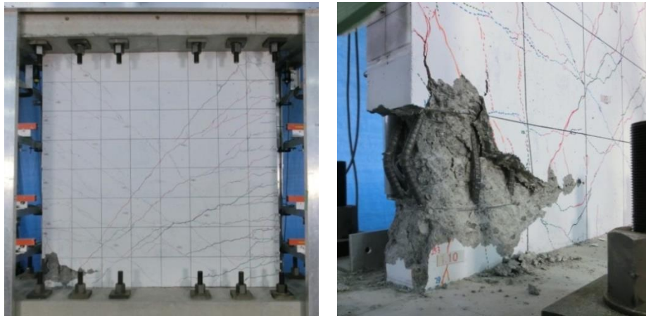
Figure 4-22 Failure of specimen WD
