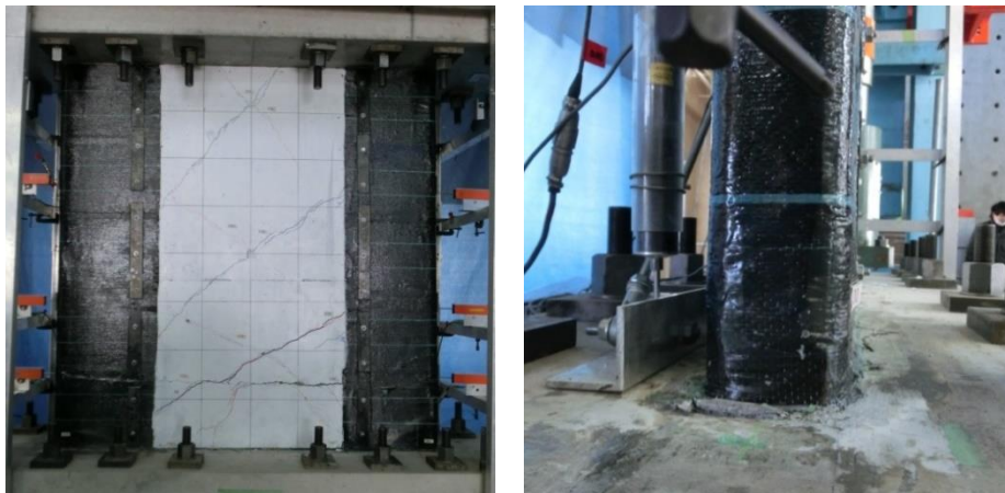
Figure 4-12 Failure of specimen RWF2
