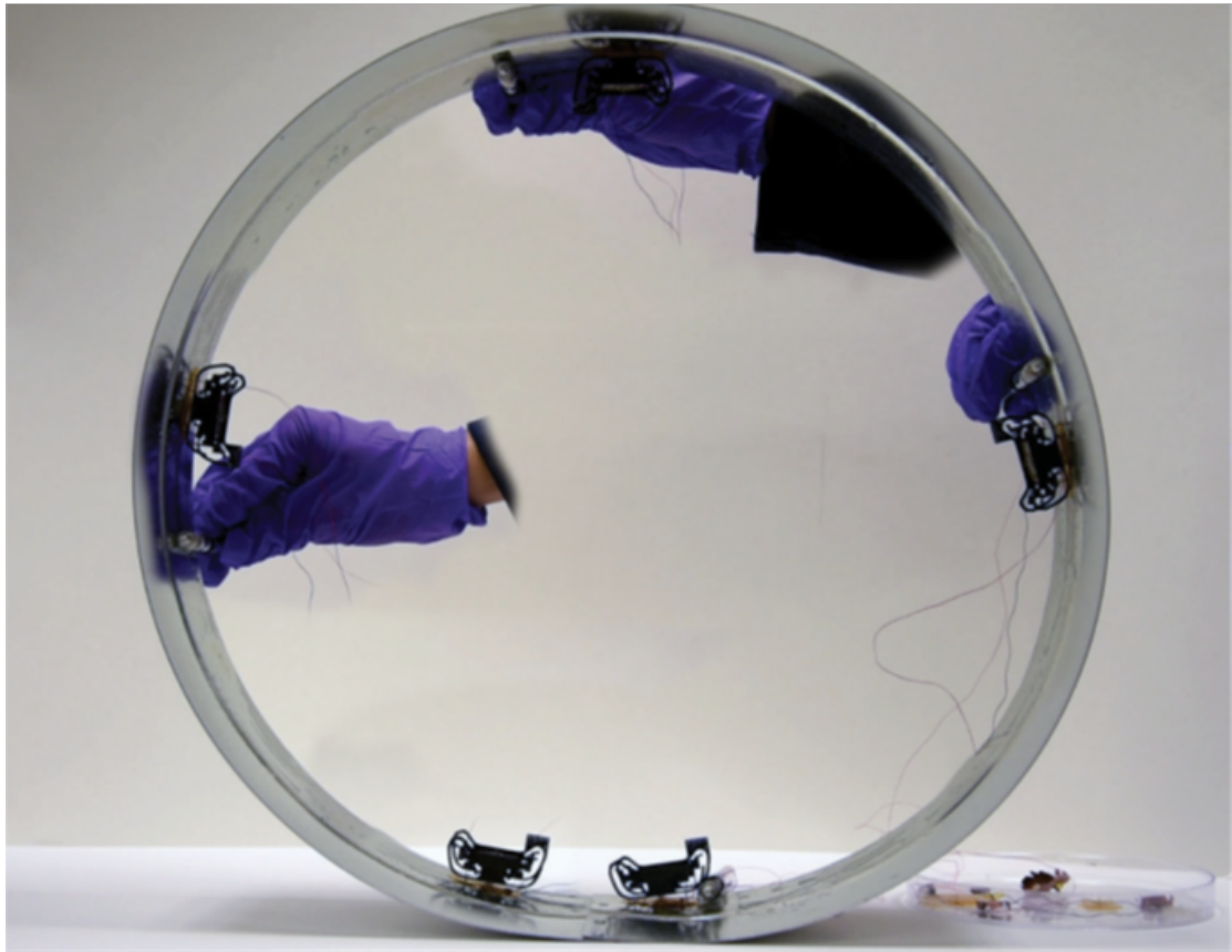
FIGURE 4.11: A 1.4 grams insect-scale prototype navigates a circular track by using capillary wet adhesion. [157]
