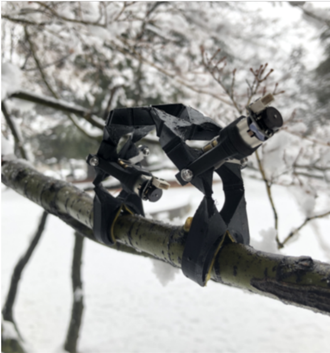
FIGURE 4.8: The Brachiation robot using elastic energy stored in its soft body and mechanical grippers to climb tree branches [143]
