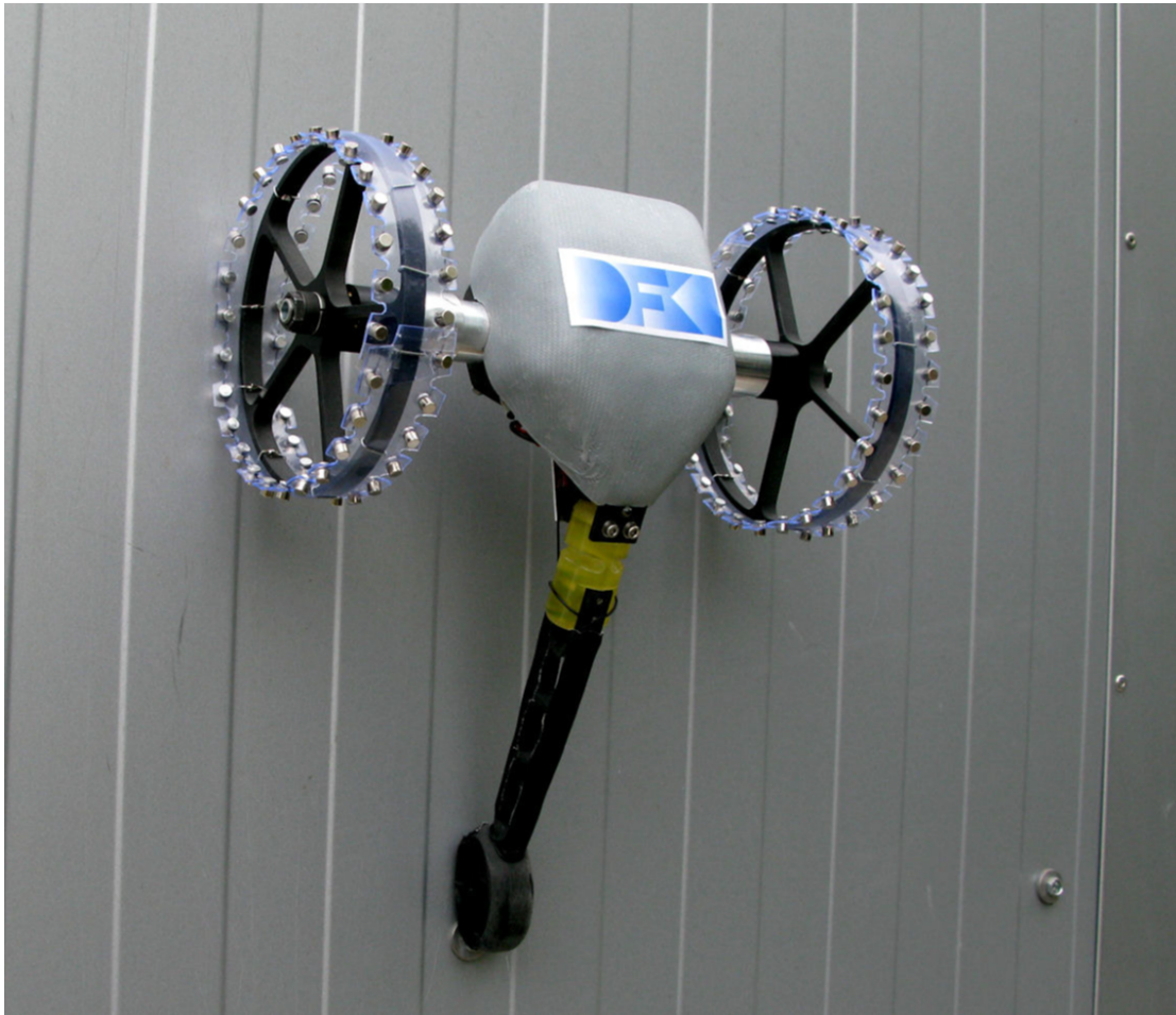
FIGURE 4.3: The MINOAS magnetic crawler uses permanent magnets on the wheels and on the tails to climb vertical walls. [127]
