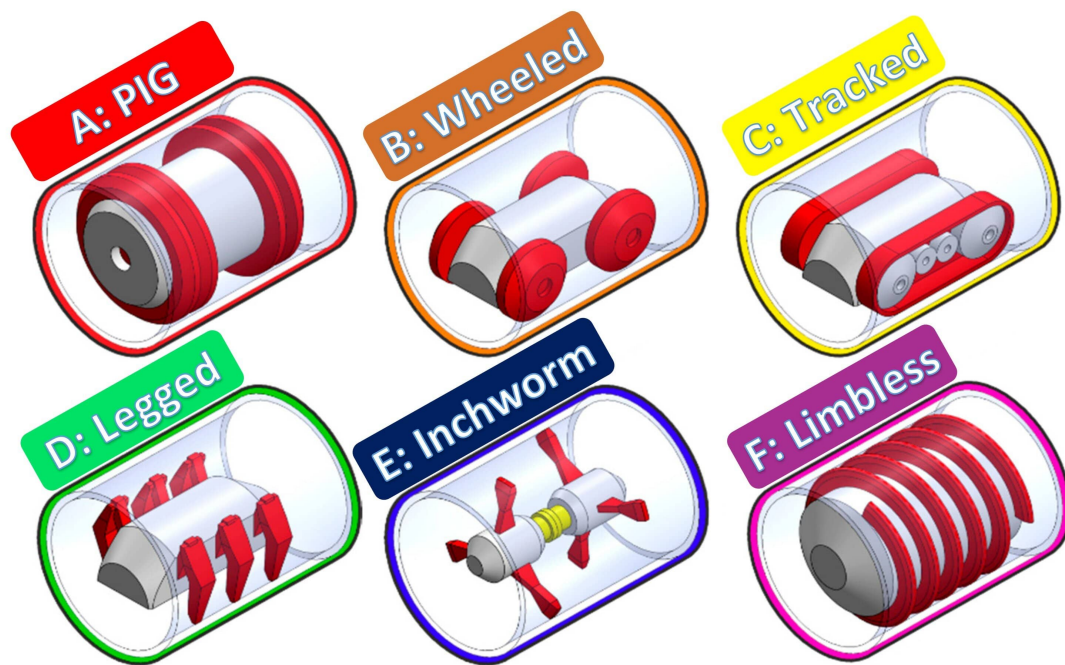
FIGURE 1.2: The main mobility mechanisms for in-pipe inspection robots previously reported. [11]
