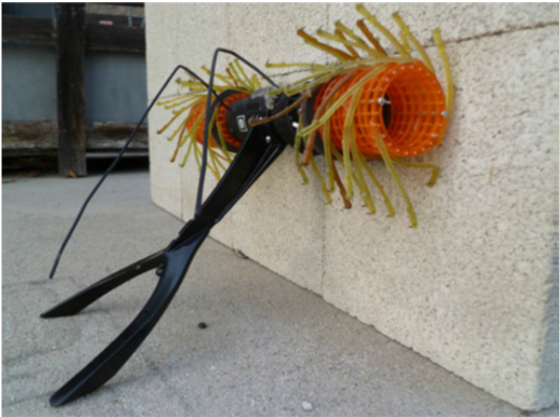
FIGURE 4.7: Recon Scout XT robot uses rotary microspine wheels to achieve advanced mobility like stair climbing and curb mounting on rough surfaces. [142]
