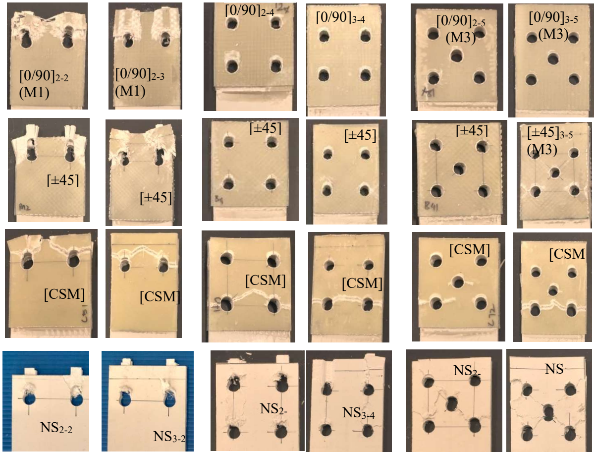
Figure 3.12 The failure obtained after the experiment in all specimens.
