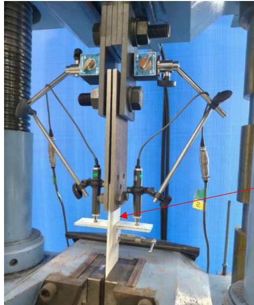
Figure 5.3 Test setup with tightening force applied in the bolted connection
