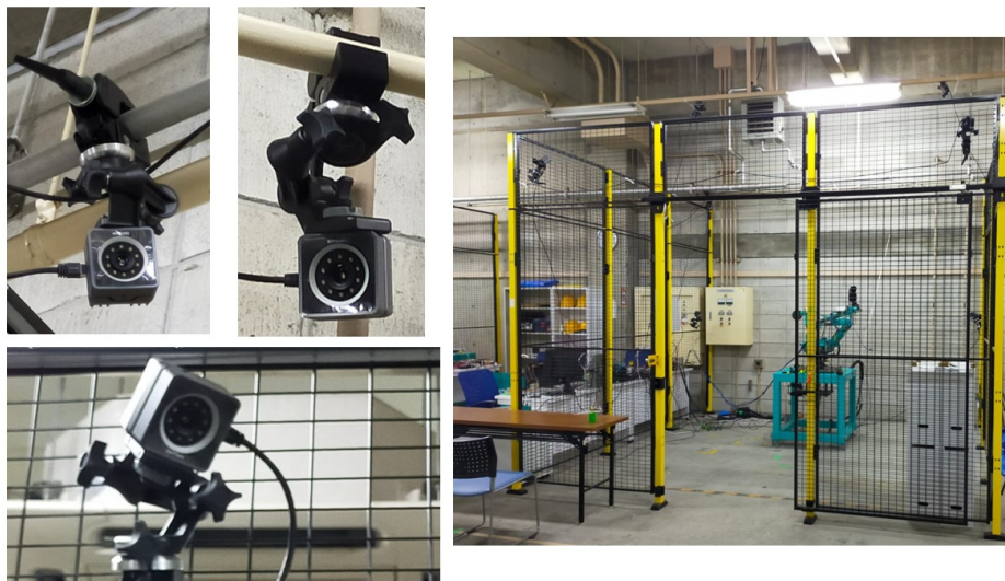
Fig. 5.8 Motion capture system attached to crane environment.
