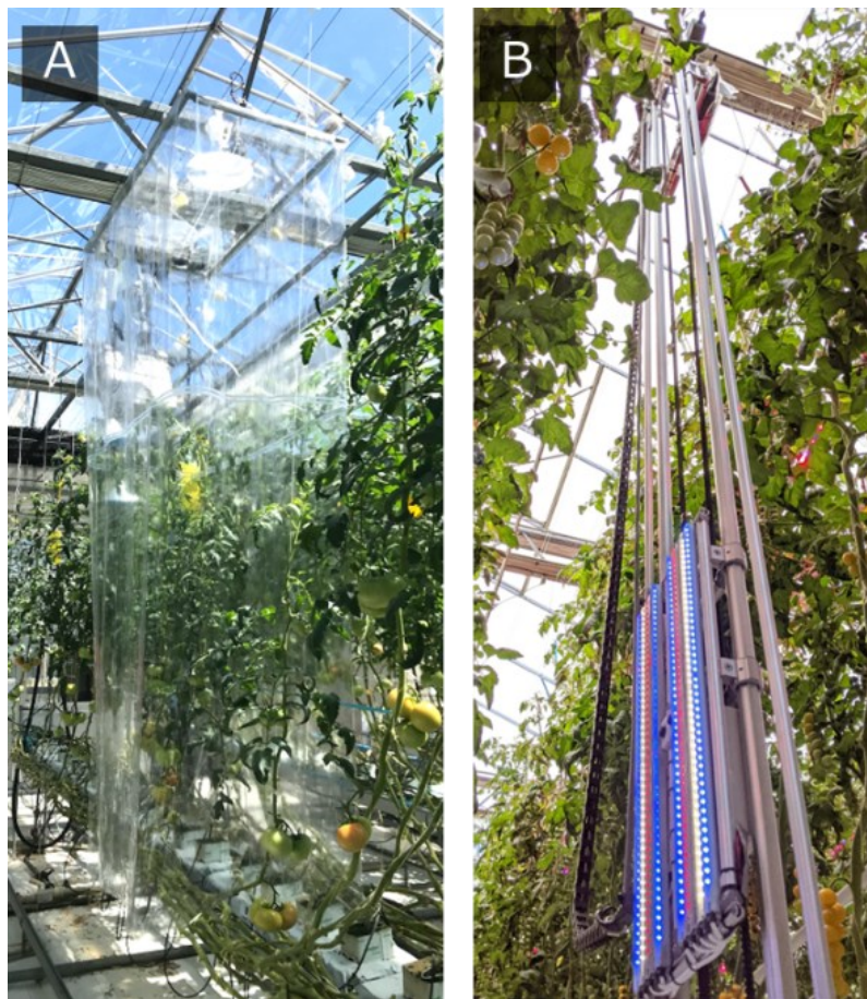
Figure 1-4: Photographs of open chamber for real-time monitoring photosynthesis(A) and hanging-type imaging robot(B).
