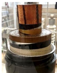
Fig. 2.1 Oil Filled HVDC Cable.
