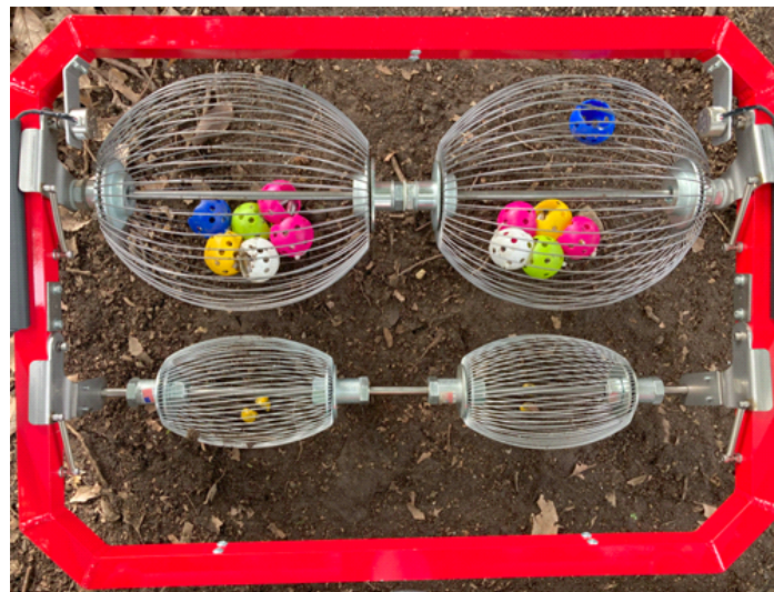
Fig. 3.10 Experimental collecting results in outdoor environment ©Fuji Technology Press Ltd., reprinted with permission from Journal of Robotics and Mechatronics.
