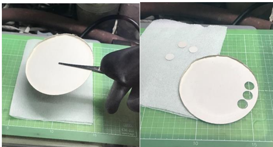
Fig. 5.1.1 Left image: Photograph of 80-mm-diameter argyrodite SE sheet after drying at 150 °C. Right image: Disks punched out from the larger sheet. The weight of each 10-mm-diameter punched-out disk was 5.6 mg, and the thickness was 61 \mu\text{m} after pressurization at 255 MPa. The ionic conductivity was 0.42 \text{mS cm}^{-1} at 25 °C.
