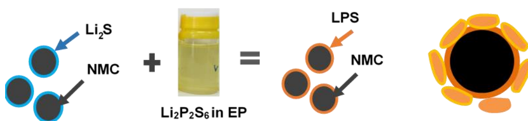
Fig. 3.1.1 The concept of the preparation procedure of NMC-LPS composite by the SEED method. NMC: \text{LiNi}_{1/3}\text{Mn}_{1/3}\text{Co}_{1/3}\text{O}_2 , EP: ethyl propionate, LPS: \text{Li}_3\text{PS}_4 .
