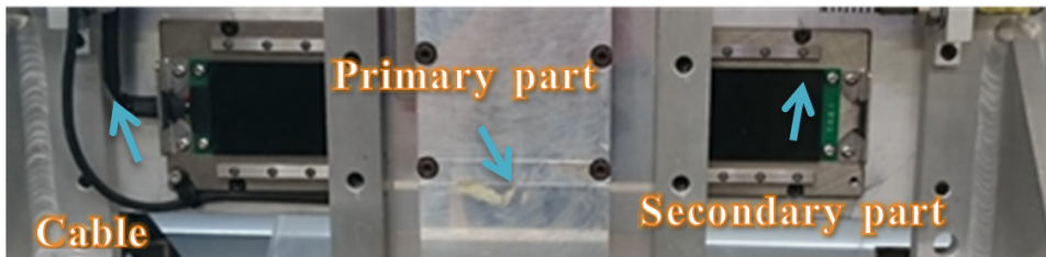
FIGURE 1.6: Direct drive - linear motor
