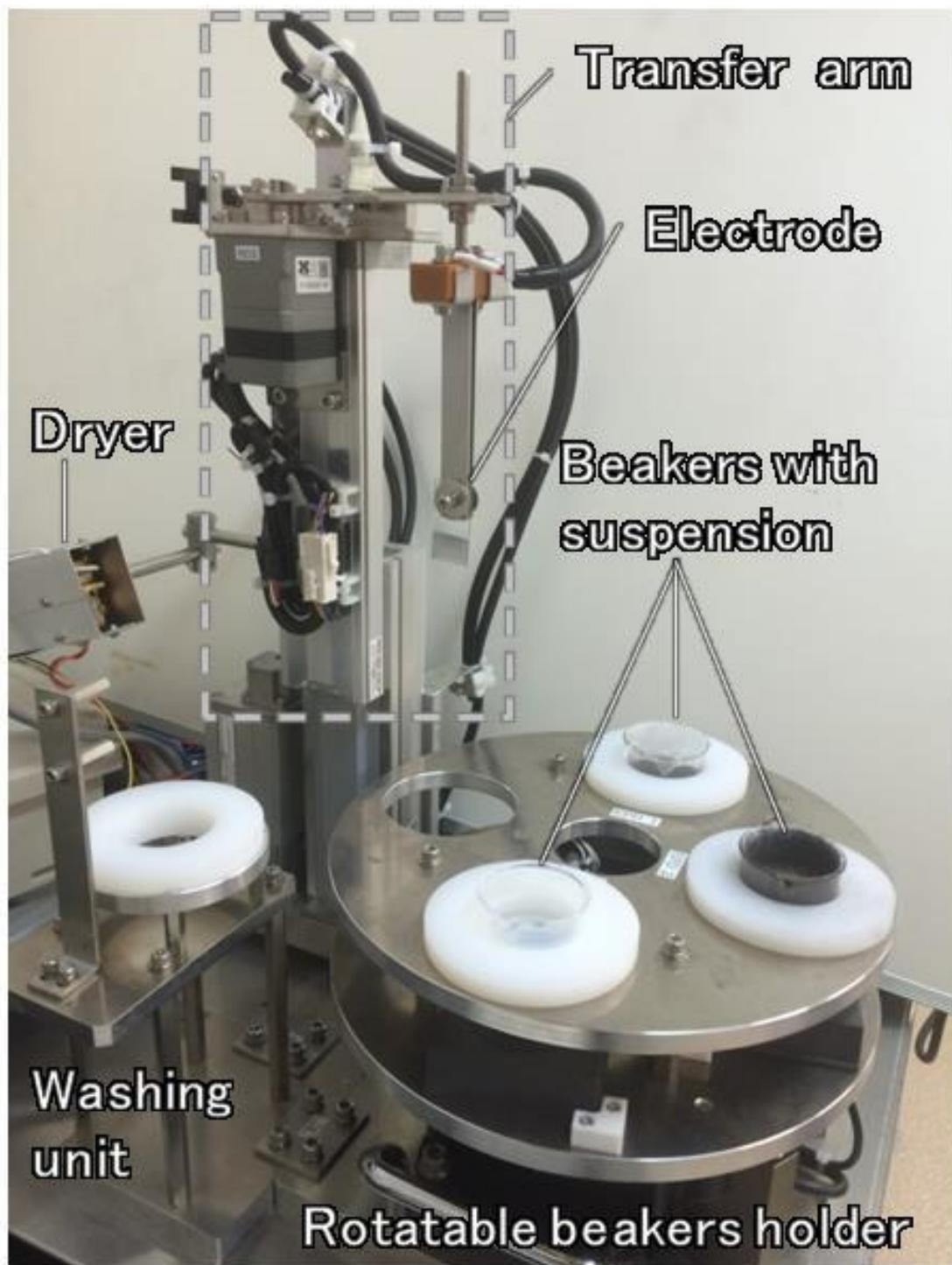
Fig. 2-1. Photograph of main unit of the EPD system.
