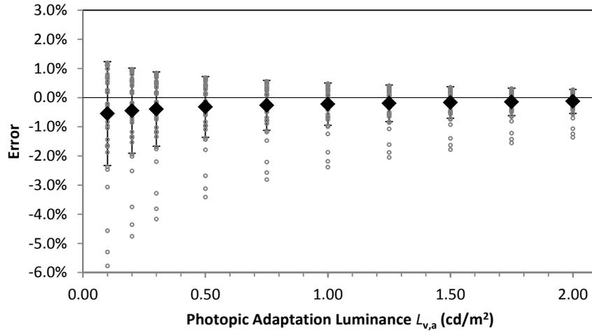
**Figure 6.7:** Simulated error distribution for the Adaptation SPD method with LED lighting. All symbols are the same as in Figure 6.5
