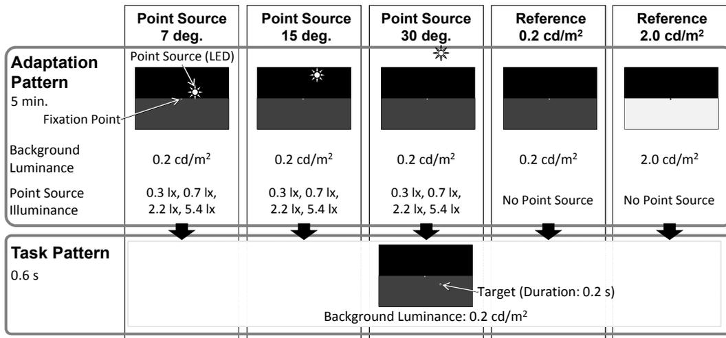
**Figure 4.2:** Adaptation patterns and a task pattern used for the point-source intensity experiment. The top row shows the adaptation patterns, and the bottom row shows the task pattern, for each condition
