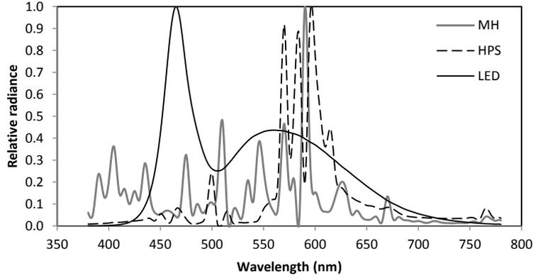
**Figure 6.4:** The SPDs of the light sources used in the error simulation
