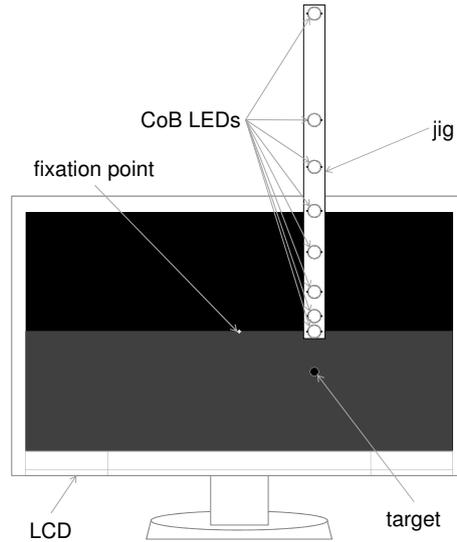
**Figure 4.4:** Schematic elevation of the LEDs, the jig and the LCD for the point-source position experiment
