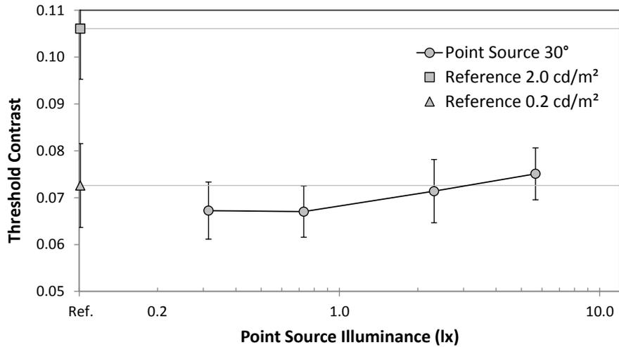
**Figure 4.9:** The mean luminance contrast detection thresholds for all subjects for a point-source position of  $30^\circ$  in the point-source intensity experiment
