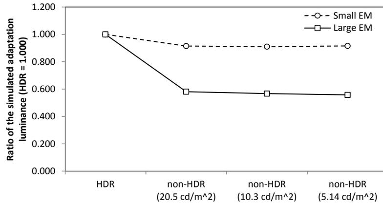
**Figure 5.8:** Ratio of the simulated adaptation luminance for non-HDR LD to that for the HDR LD. The simulations were done with the large EM and the small EM
