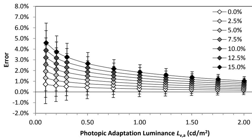
**Figure 6.13:** Simulated errors in the mesopic luminance calculated with the Source SPD method in some adaptation fields illuminated with LEDs and HPS. Each symbol shows a different HPS ratio (0 % to 15 %) in the adaptation field mainly lit by LEDs. The error bars show one standard deviation of the errors
