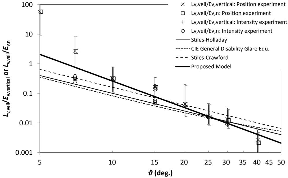
**Figure 4.14:** The surrounding luminance effects from the experiments (symbols) and the veiling luminance predicted with the models (lines), per one lux of vertical or normal illuminance from the point source
