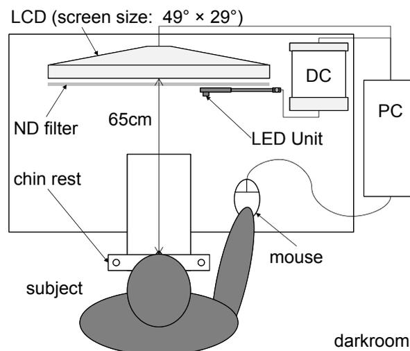
**Figure 4.1:** Depiction of the set-up for the point-source intensity experiment
