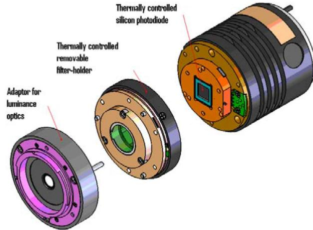
**Figure 2.2:** A physical detector of optical radiation, NIST working standard detector. (NIST Technical Note 1621 [13])
