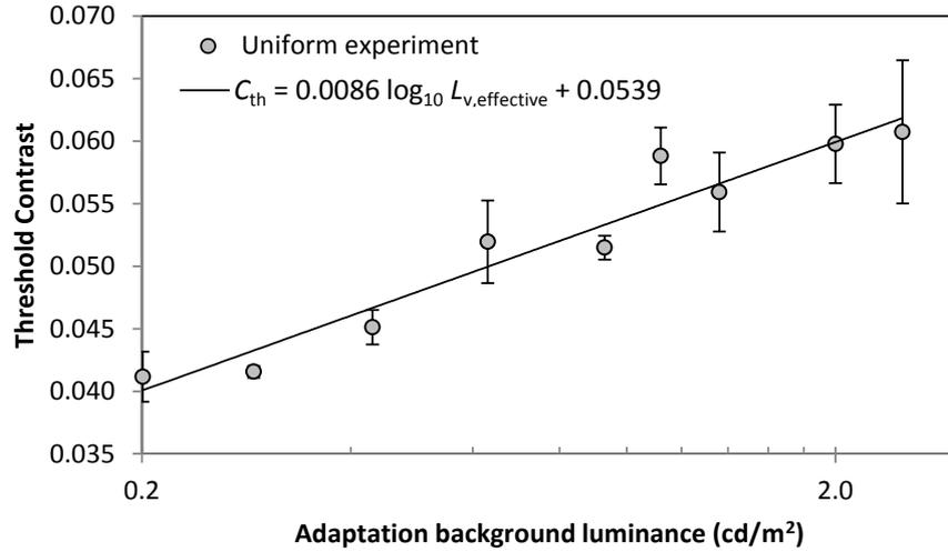
**Figure 4.12:** The mean luminance contrast detection thresholds for repeated trials with one subject in the uniform experiment
