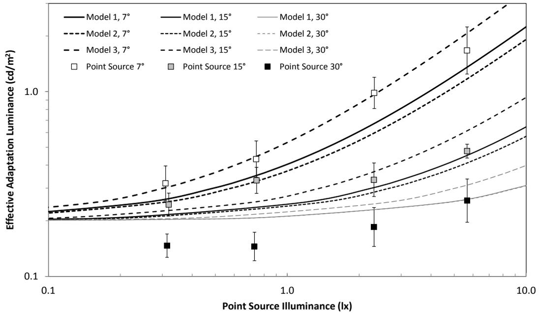
**Figure 4.13:** The effective adaptation luminances determined from the experimental results and the models, as functions of the vertical illuminance from the point source. Square symbols show the experimental results; white, grey, and black correspond to 7°, 15°, and 30°, respectively. Lines show the effective adaptation luminance from the models; solid, short dashed, and long dashed lines correspond to the Models 1, 2, and 3, respectively
