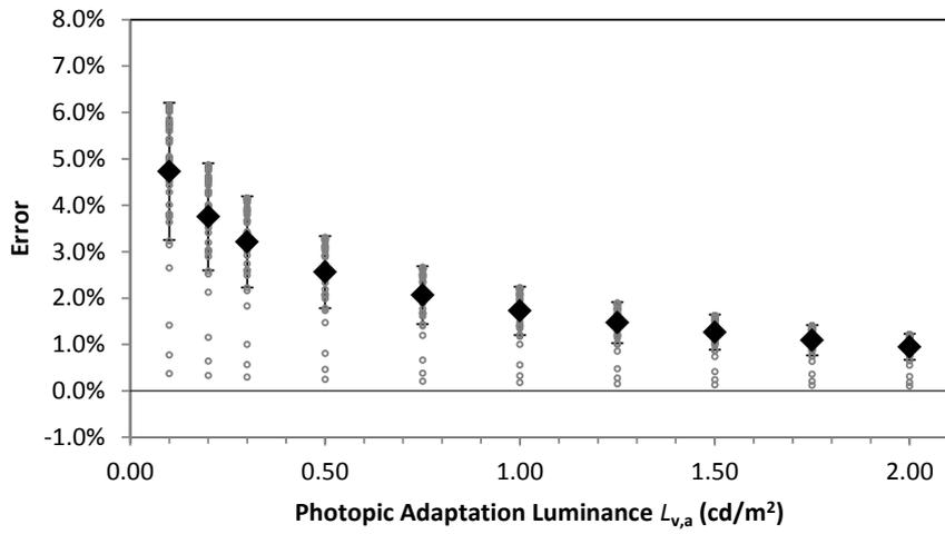
**Figure 6.8:** Simulated error distribution for the Source SPD method with MH lighting. All symbols are the same as in Figure 6.5
