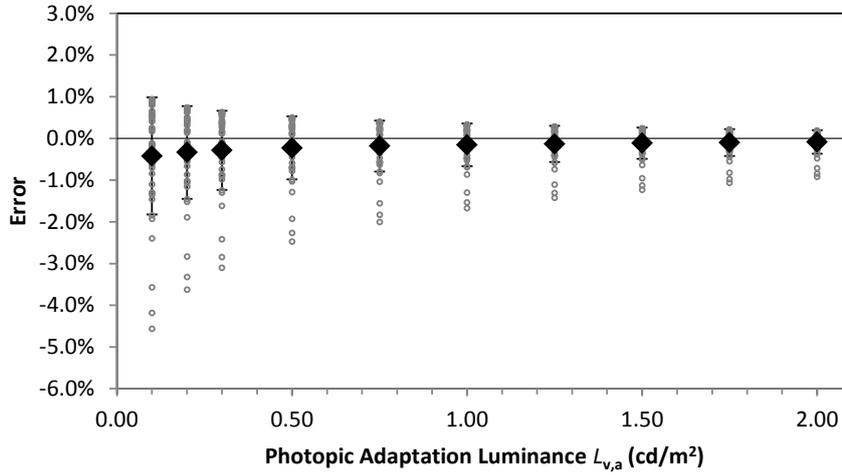
**Figure 6.5:** Simulated error distribution for the Adaptation SPD method with MH lighting. The small gray circle symbols show the errors for each test point. The filled diamond symbols show the average error at each photopic adaptation luminance. The error bars are one standard deviation
