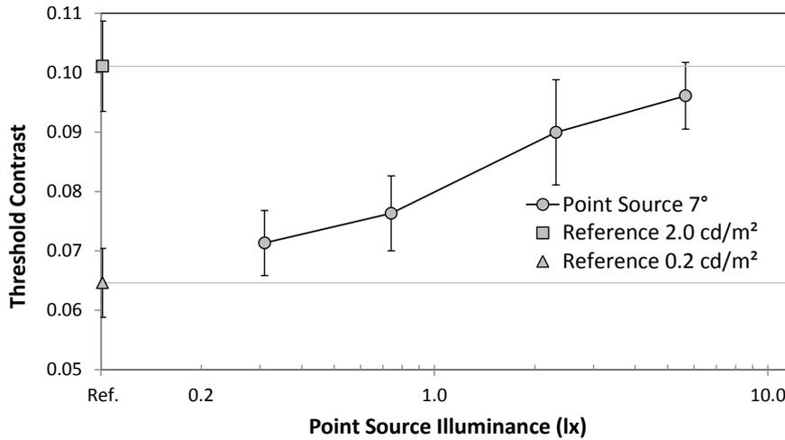
Figure 4.7: The mean luminance contrast detection thresholds for all subjects for a point-source position of 7° in the point-source intensity experiment
