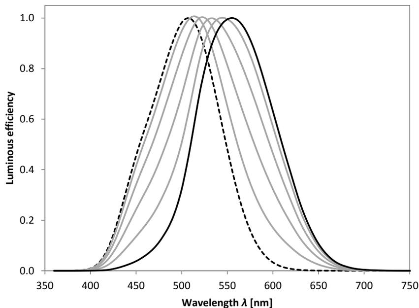
**Figure 1.1:** Spectral luminous efficiency functions. The black solid line and the black dash line show the photopic spectral luminous efficiency function  $V(\lambda)$  and the scotopic spectral luminous efficiency function  $V'(\lambda)$ , respectively. The gray lines show some mesopic spectral luminous efficiency functions  $V_{\text{mes};m}(\lambda)$  with various adaptation coefficient,  $m$
