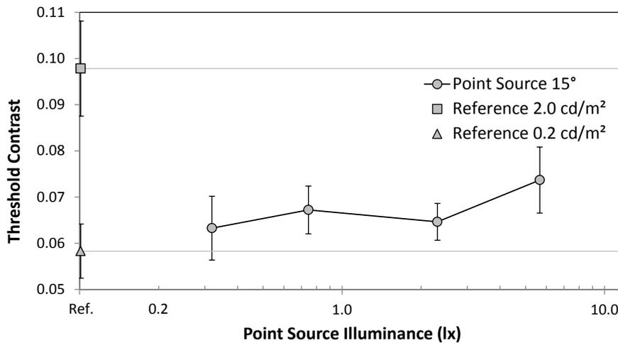
Figure 4.8: The mean luminance contrast detection thresholds for all subjects for a point-source position of 15° in the point-source intensity experiment
