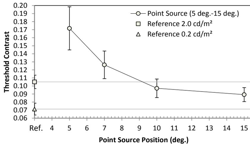
**Figure 4.10:** The mean luminance contrast detection thresholds for all subjects for the near-point-source conditions and associated reference conditions in the point-source position experiment
