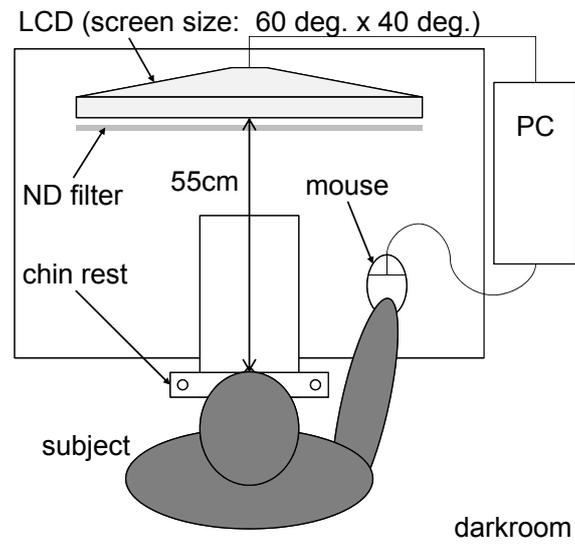
**Figure 3.1:** Depiction of the experimental set-up for the adaptation pattern experiment and the adaptation background luminance experiment
