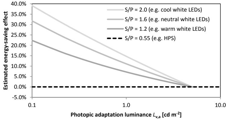
**Figure 2.7:** Estimated energy-saving effect by lighting design with the mesopic photometry system. An S/P ratio of 0.55, which represents HPS, was chosen as reference
