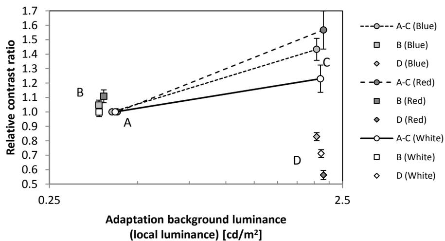
**Figure 3.5:** The mean luminance contrast detection thresholds normalized for the Condition A thresholds in adaptation pattern experiment. Each symbol shows the same type of data as in Figure 3.4
