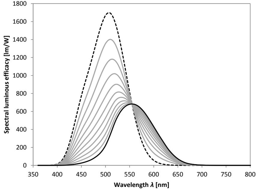
**Figure 2.6:** The mesopic spectral luminous efficacy functions. The function with  $m = 1$  (black solid line) and with  $m = 0$  (black dashed line) are the same as  $K(\lambda)$  and  $K'(\lambda)$ , respectively
