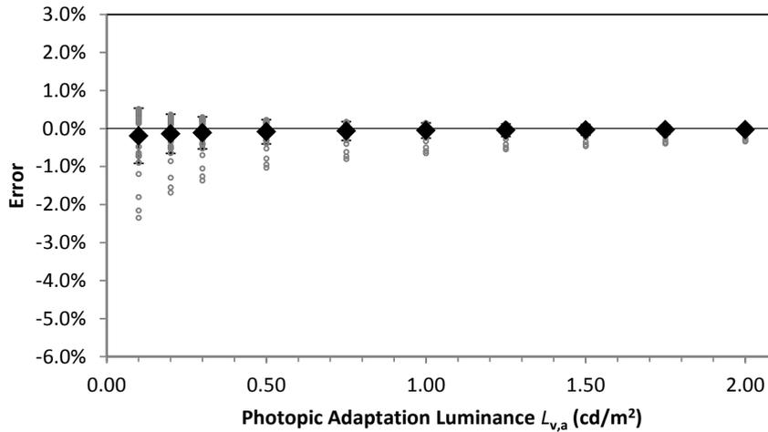
**Figure 6.6:** Simulated error distribution for the Adaptation SPD method with HPS lighting. All symbols are the same as in Figure 6.5
