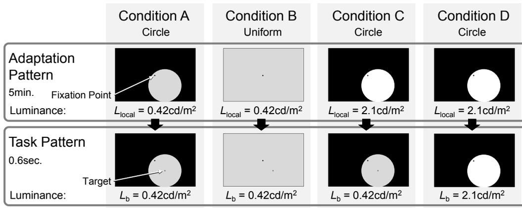
**Figure 3.3:** Adaptation patterns and task patterns used for the adaptation pattern experiment. The top row shows the adaptation patterns, and the bottom row shows the task patterns, for each Condition A to D. The circular illuminated area of the adaptation pattern for Condition C is 20 % of the entire screen illuminated for Condition B, and the luminance is five times higher than that for Condition B. Thus, the mean luminances of the adaptation pattern for Conditions B and C are nearly equal
