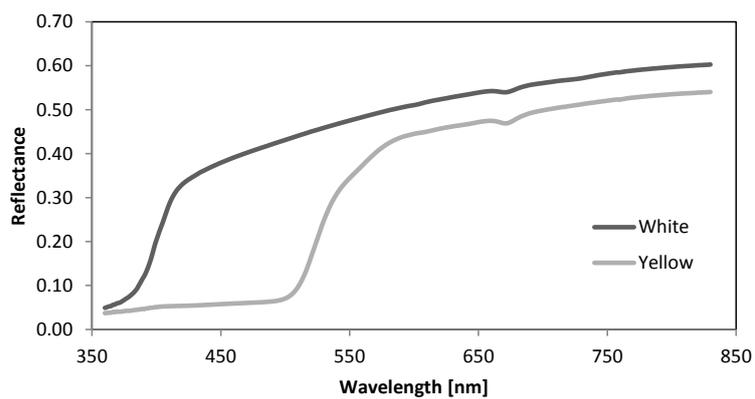
Figure 6.3: The spectral reflectance of fresh yellow and white paint on a road
