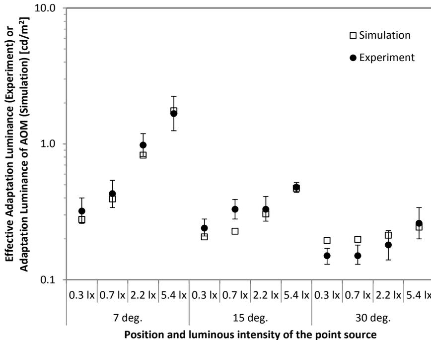
**Figure 5.2:** Comparisons of the simulated adaptation luminance and the effective adaptation luminance in the point-source intensity experiment
