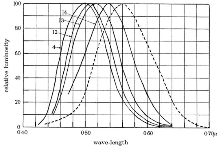
**Figure 2.5:** Mesopic spectral luminous efficiency at  $10^\circ$  eccentricity (Walters and Wright, 1942 [31])
