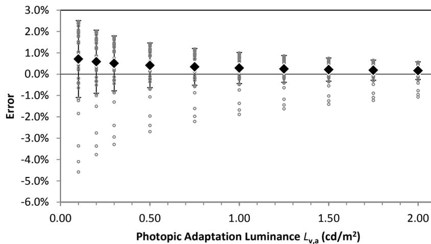
**Figure 6.12:** Simulated error distribution for the corrected Source SPD method with LED lighting. The source S/P ratio was corrected with the correction factor (= 0.898). All symbols are the same as in Figure 6.5
