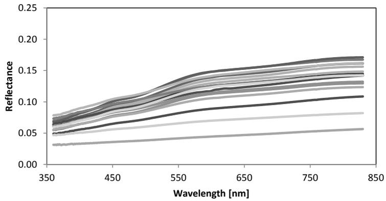
Figure 6.1: The spectral reflectance of road surfaces in good condition
