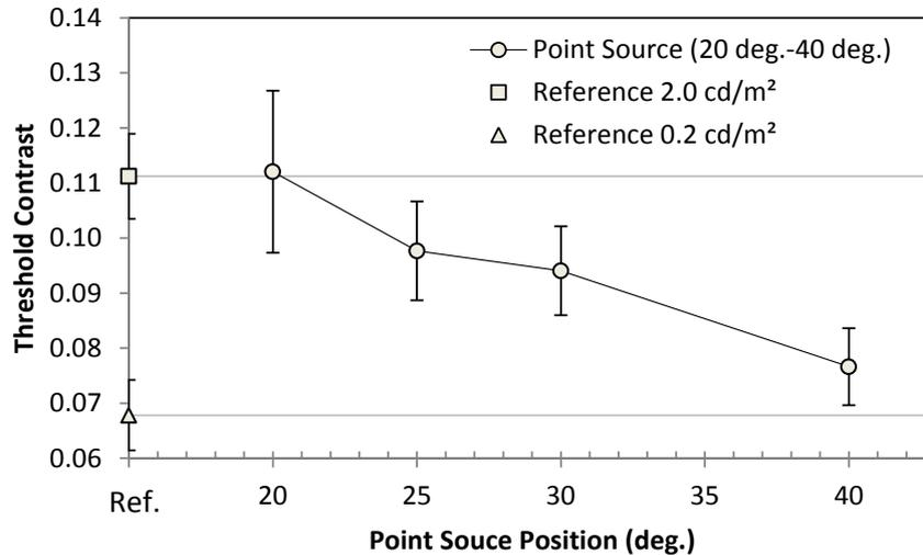
**Figure 4.11:** The mean luminance contrast detection thresholds for all subjects for the far-point-source conditions and associated reference conditions in the point-source position experiment
