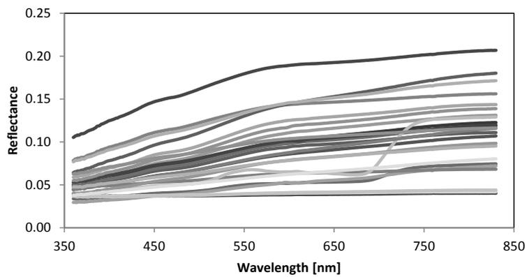
Figure 6.2: The spectral reflectance of damaged road surfaces
