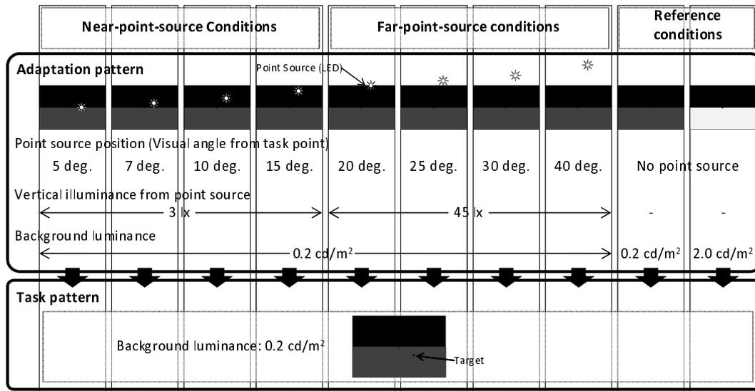
**Figure 4.5:** Adaptation patterns and a task pattern used for the point-source position experiment
