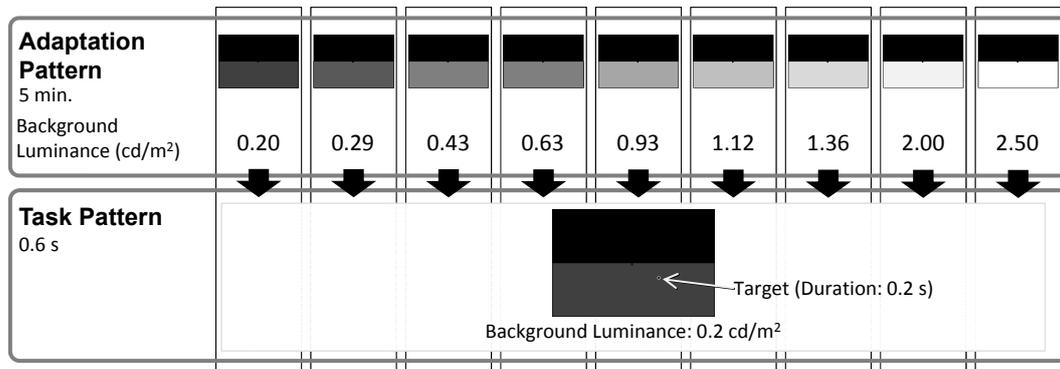
**Figure 4.6:** Adaptation patterns and a task pattern used for the uniform experiment
