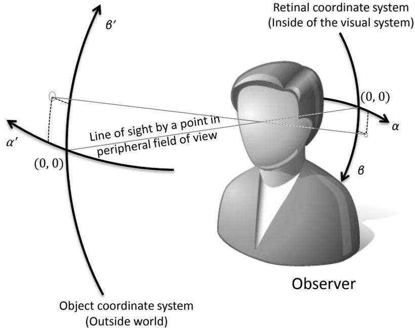
**Figure 5.1:** The object coordinate system and the retinal coordinate system. Both coordinate systems share a pivot at the observer's eye position
