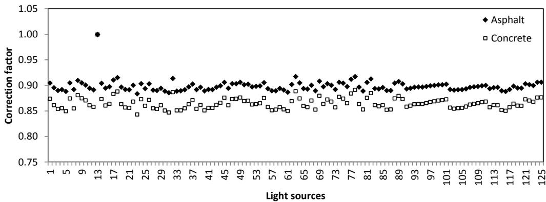
**Figure 6.11:** Correction factors for various light sources with spectral reflectance data of asphalt and concrete
