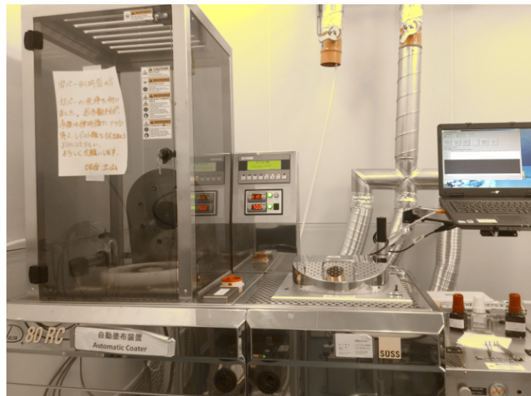
Figure 2.14: Suss Delta80 spin-coater with hotplate. Photograph: Clean Room, Toyohashi University of Technology
