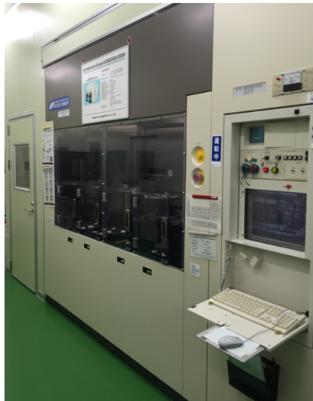
Figure 2.21: Ion implantation system EXCEED2300/2300H. Photograph: Clean Room, Toyohashi University of Technology
