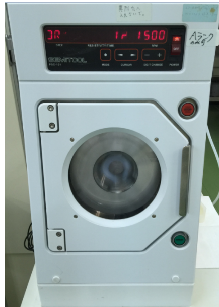
Figure 2.17: A spin dryer while operating for 2 inch wafers. Photograph: Clean Room, Toyohashi University of Technology
