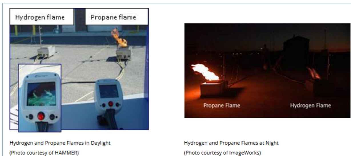
Figure 1.2: Hydrogen flame visibility in daylight (left) and at night (right) comparing with propane flame. Source: https://h2tools.org/bestpractices/h2introduction/hazards/flames
