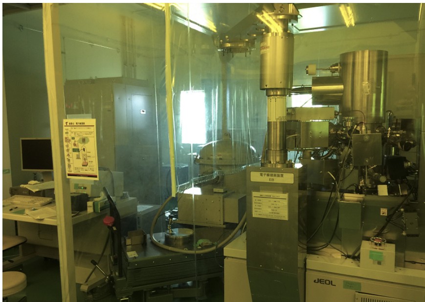
Figure 2.4: Electron-beam lithography machine JBX-6300D by Jeol Ltd. Photograph: Clean Room, Toyohashi University of Technology
