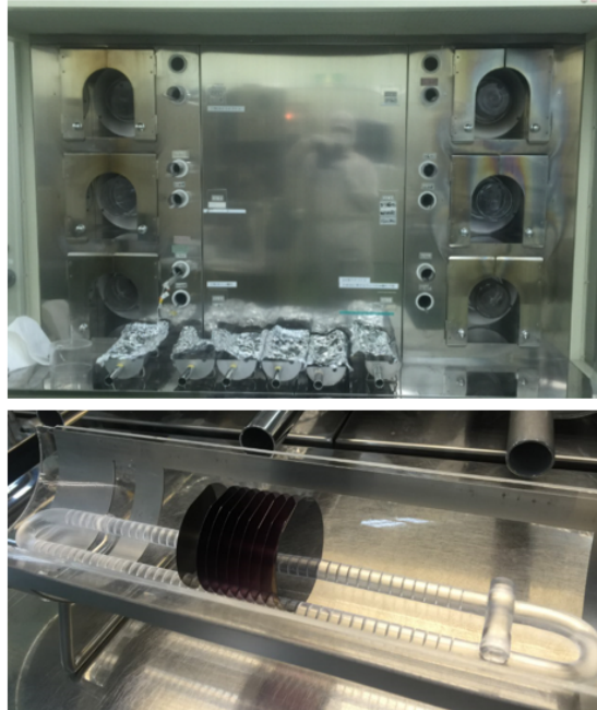
Figure 2.7: Oxidation furnace. (top) Six furnaces for different use and temperature. (bottom) Wafers are loaded in the quartz boat. Photograph: Clean Room, Toyohashi University of Technology
