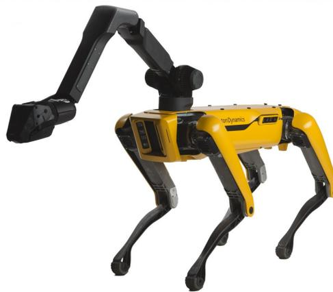
Fig. 1.2 SpotMini developed by Boston Dynamics [11]. It weighs 25 kg (30 kg including the 5 degree-of-freedom arm) and driven by batteries lasting for 90-minute operation time on a charge. It has perception sensors including stereo cameras, depth cameras, an inertia measurement unit, and position/force sensors in the limbs.
