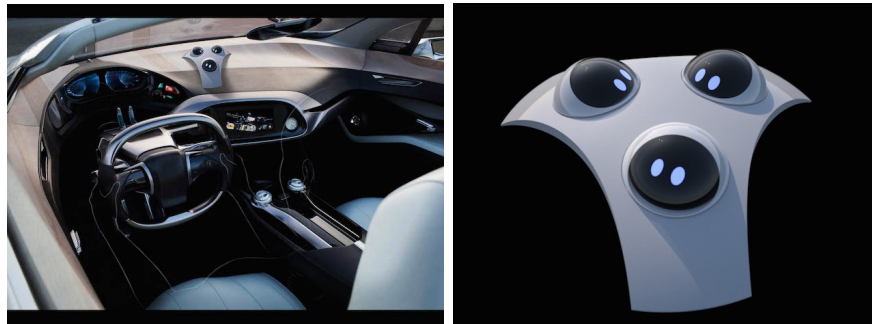
Figure 2-3: Base unit of NAMIDA, designed to be secured on the dashboard of the car within the peripheral vision of the driver ( left ). With movable heads and eyes, NAMIDA projects a life-like appearance ( right ).
