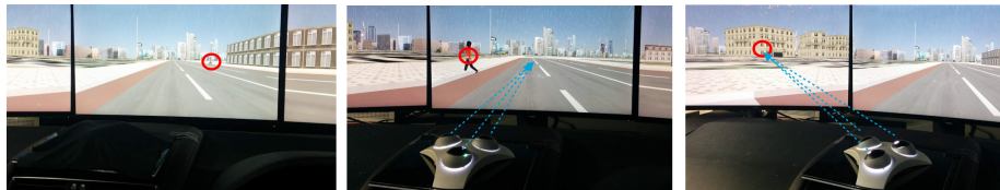
Figure 4-2: The NN ( left ), NRB ( middle ) and NFB ( right ) conditions are shown. The red circle represents the gaze point of the human operator. The blue arrows represent the gaze direction of the robots.
