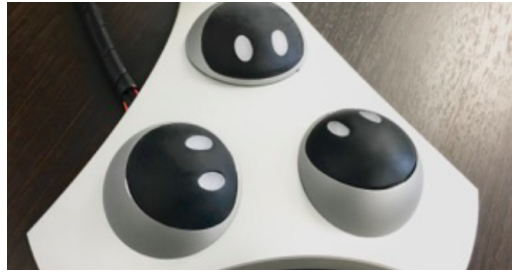
Figure 5-1: NAMIDA consists of three robots that is designed to be placed on dashboard on a car.
